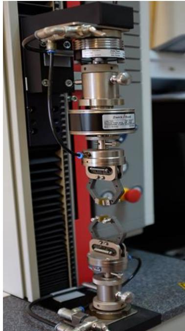
**Fig. 1.** Universal Testing Machine for fibre tensile test
