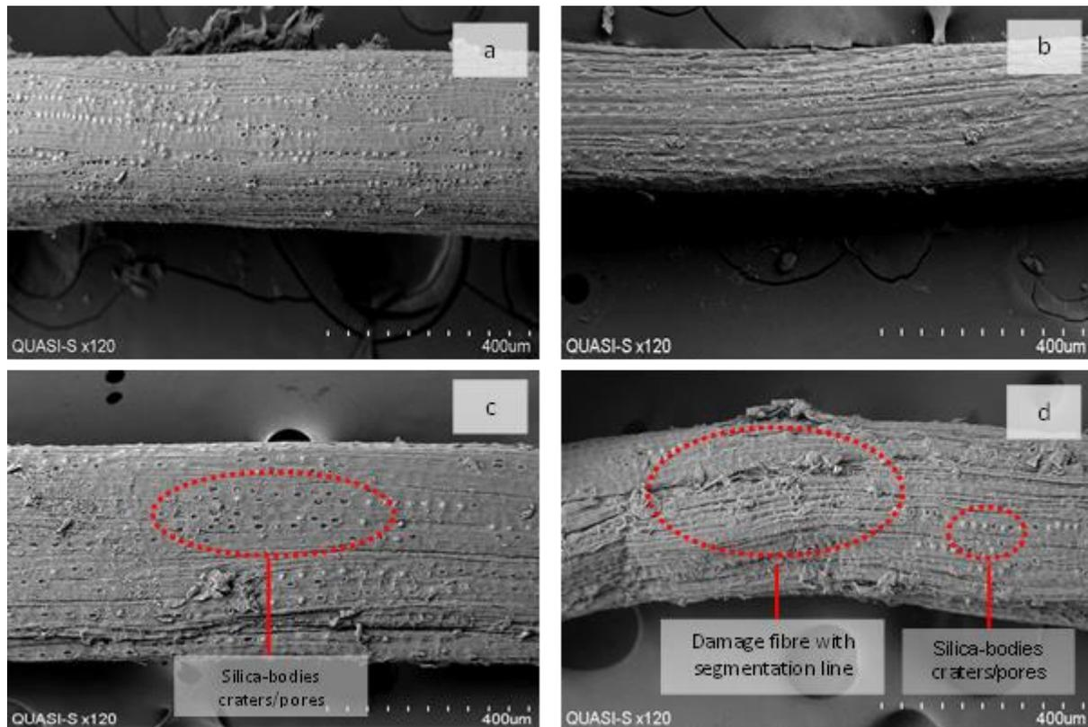
**Fig. 5.** SEM images of EFB fibre treated with (a) 0.2%, (b) 0.4%, (c) 0.6%, and (d) 0.8% acetic acid at 120x magnification
