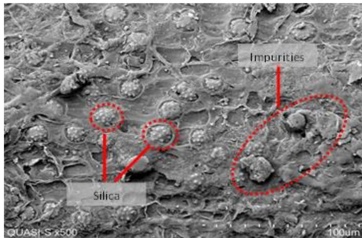
**Fig. 3.** SEM image of untreated EFB fibre at 500x magnification
