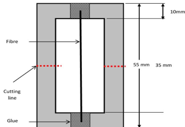
**Fig. 2.** Schematic representation of the experimental setup of tensile test
