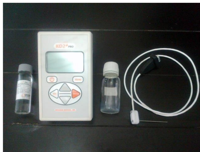
Fig. 1. KD2 Pro used to measure the thermal conductivity of nanofluid
