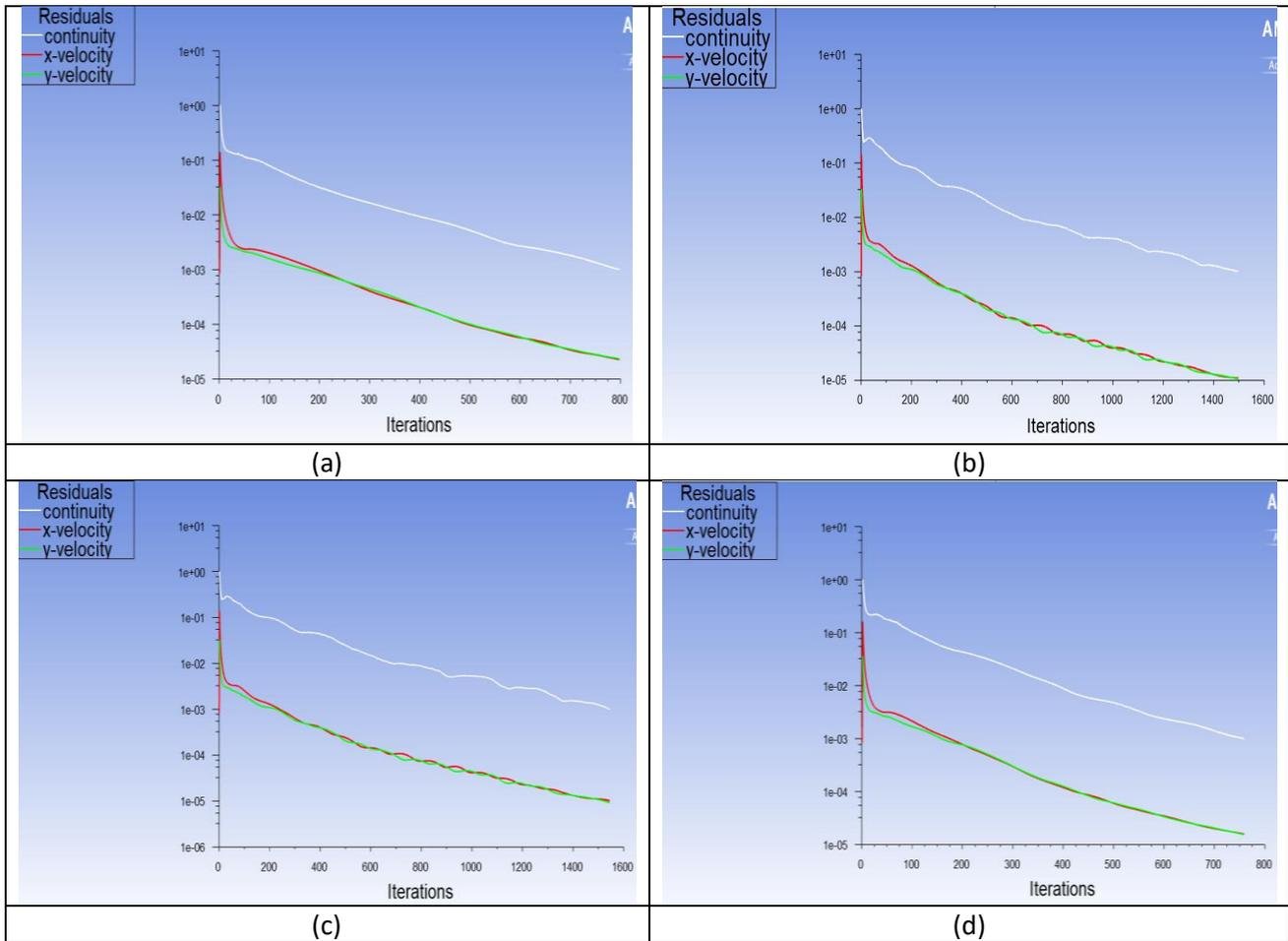
**Fig. 9.** Convergence plot at  $Re = 3200$  computed by: (a) FOU; (b) SOU; (c) QUICK; (d) power-law scheme with grid number  $129 \times 129$
