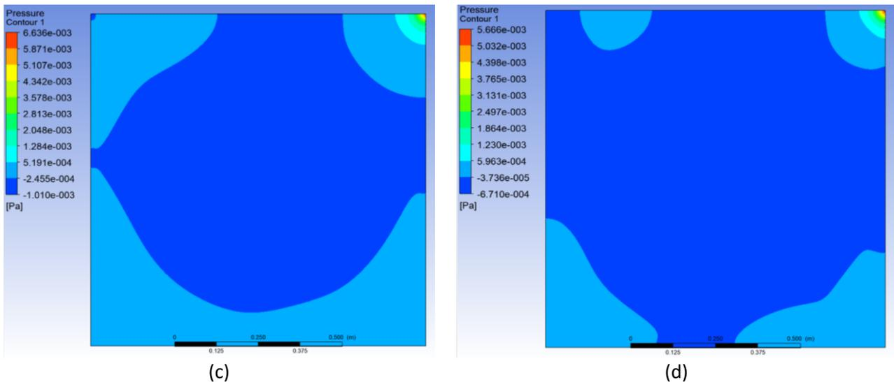
**Fig. 7.** Computed pressure field at  $Re = 3200$  computed by: (a) FOU; (b) SOU; (c) QUICK; (d) power-law scheme with grid number  $129 \times 129$
