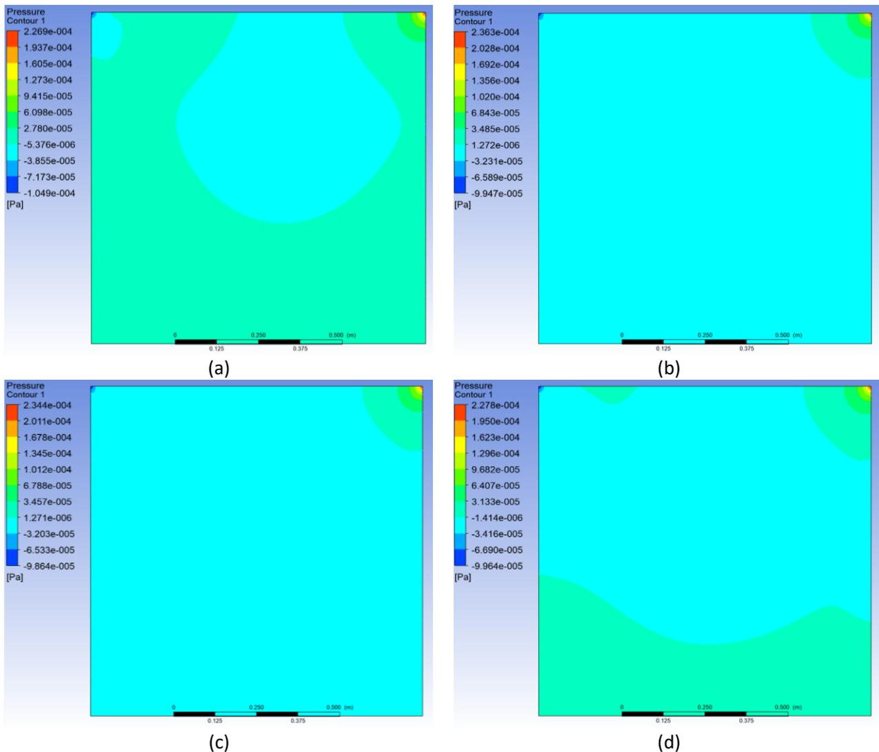
**Fig. 4.** Computed pressure field at  $Re = 400$  computed by: (a) FOU; (b) SOU; (c) QUICK; (d) power-law scheme with grid number  $129 \times 129$
