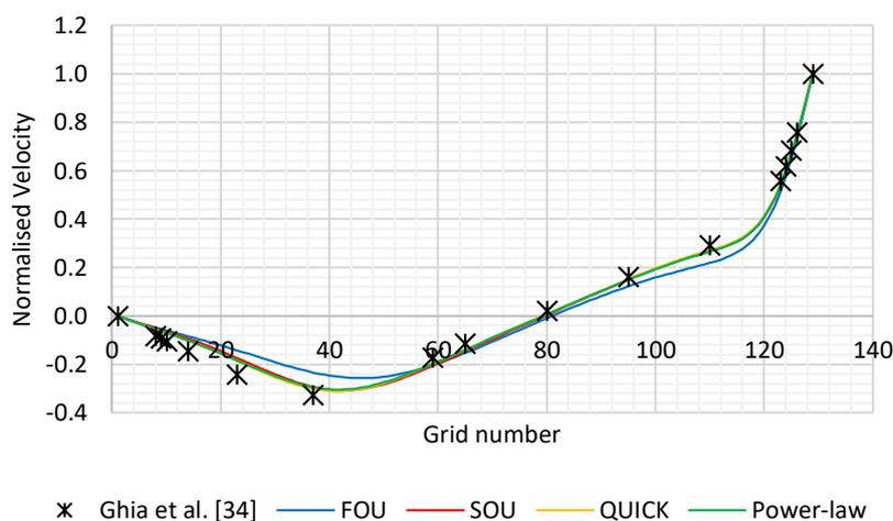
**Fig. 10.** Comparison of velocity field of  $u_x$  at the middle line of the  $x$ -axis of the lid-driven cavity at  $Re = 400$
