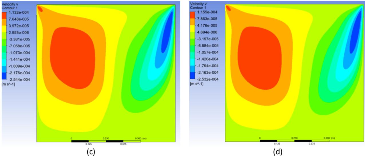
**Fig. 3.** Computed  $u_y$  field at  $Re = 400$  computed by: (a) FOU; (b) SOU; (c) QUICK; (d) power-law scheme with grid number  $129 \times 129$
