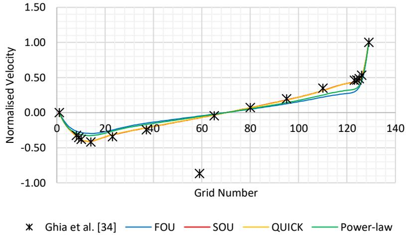
**Fig. 11.** Comparison of velocity field of  $u_x$  at the middle line of the x-axis of the lid-driven cavity at  $Re = 3200$
