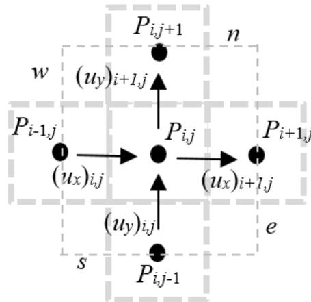
**Fig. 1.** Grid formation using staggered grid
