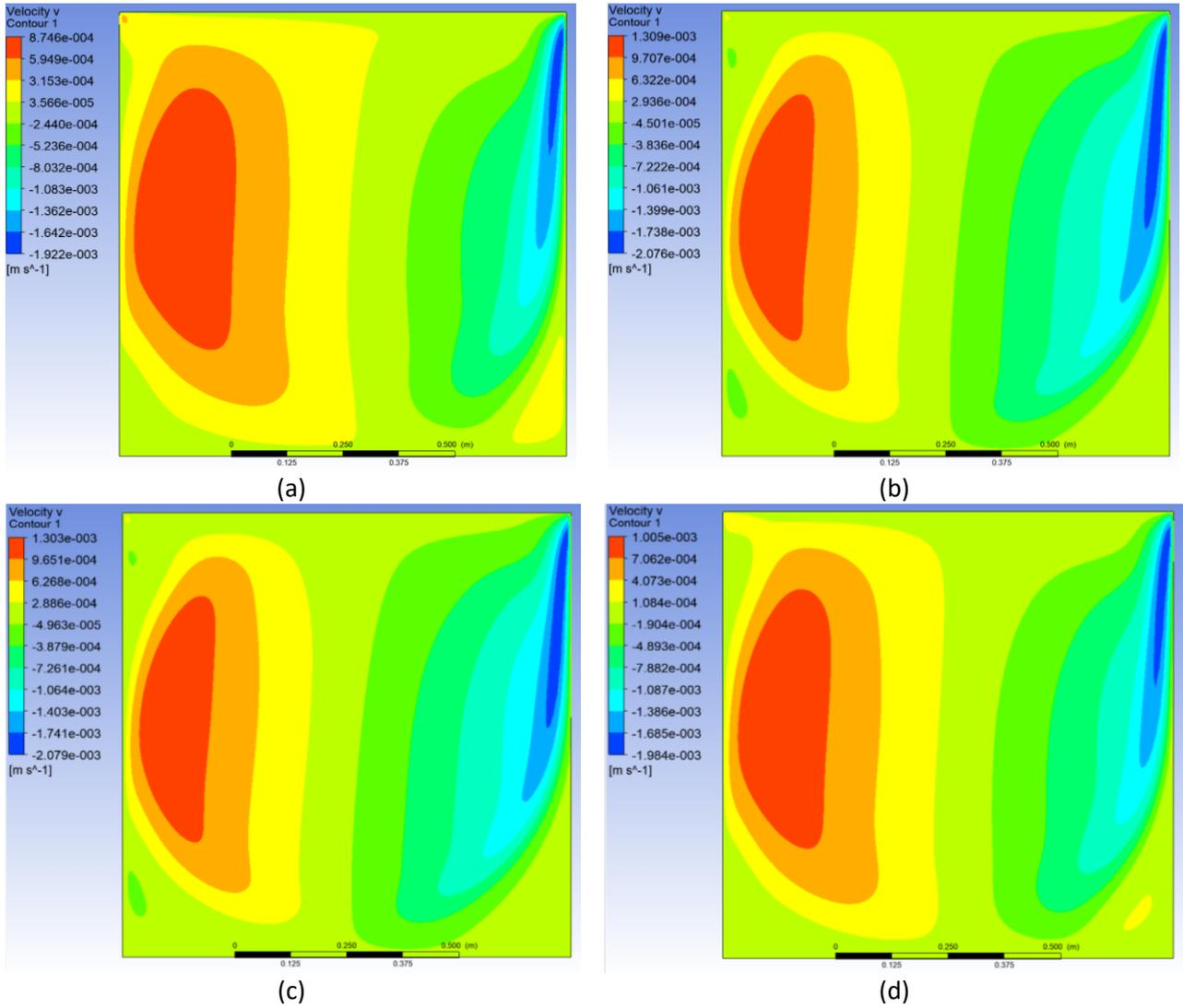
**Fig. 6.** Computed  $u_y$  field at  $Re = 3200$  computed by: (a) FOU; (b) SOU; (c) QUICK; (d) power-law scheme with grid number  $129 \times 129$
