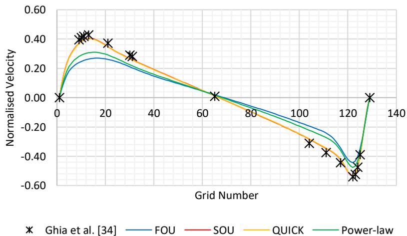
**Fig. 13.** Comparison of velocity field of  $u_y$  at the middle line of the y-axis of the lid-driven cavity at  $Re = 3200$
