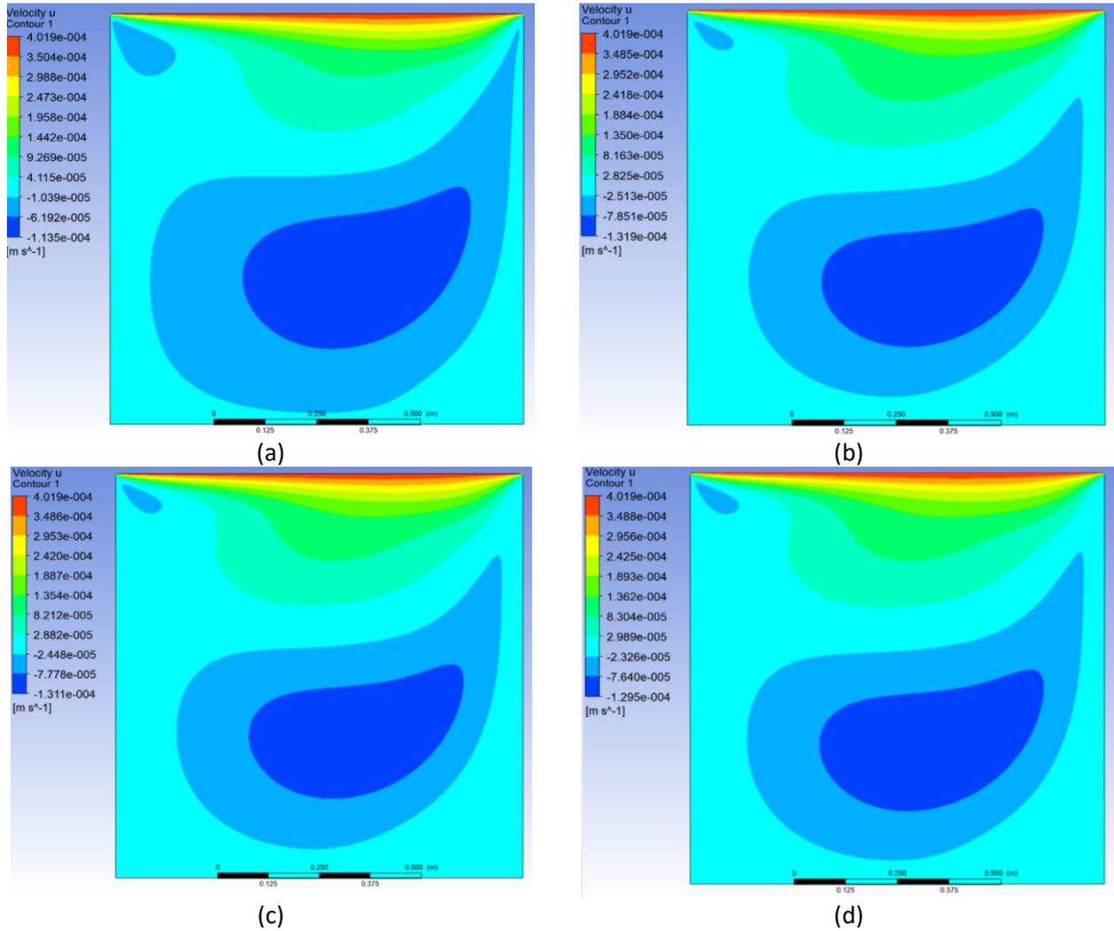
**Fig. 2.** Computed  $u_x$  field at  $Re = 400$  computed by: (a) FOU; (b) SOU; (c) QUICK; (d) power-law scheme with grid number  $129 \times 129$
