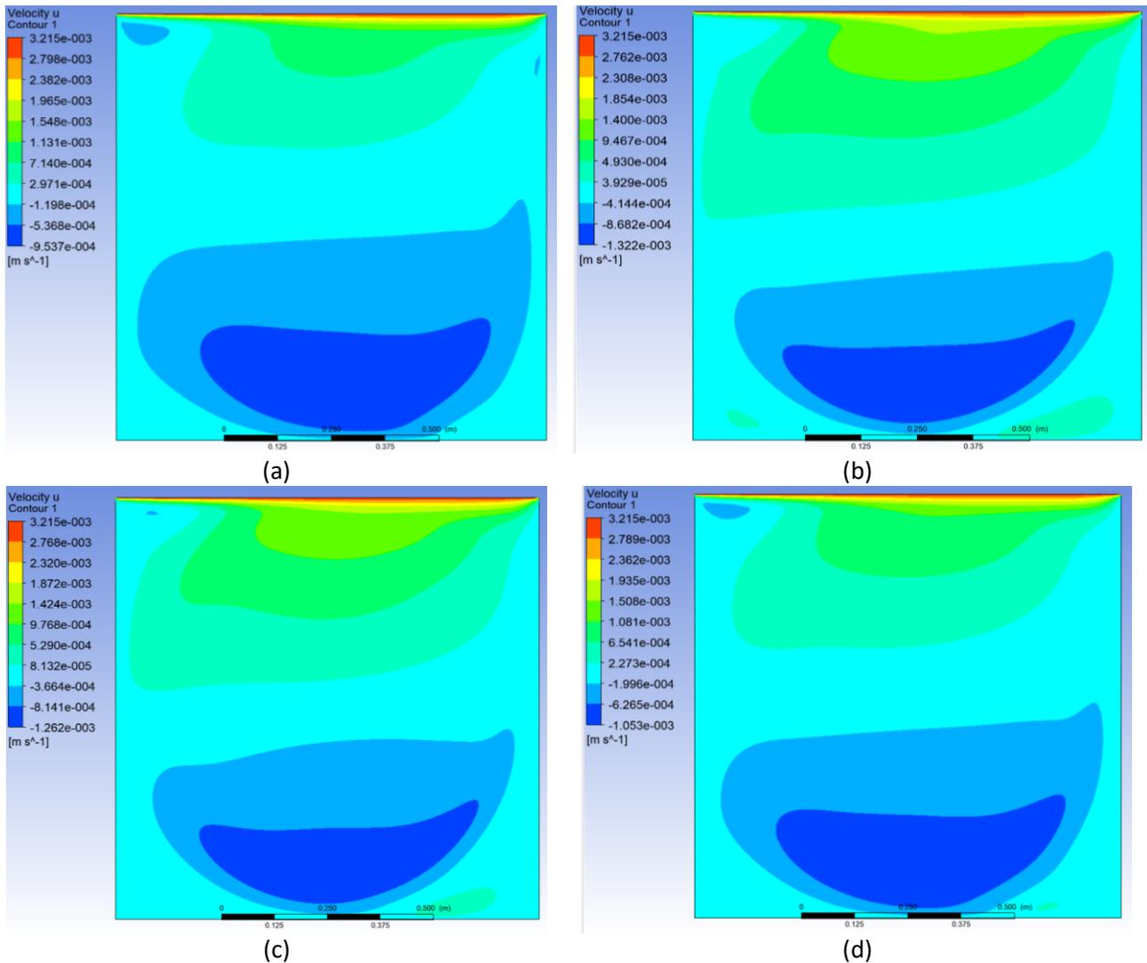
**Fig. 5.** Computed  $u_x$  field at  $Re = 3200$  computed by: (a) FOU; (b) SOU; (c) QUICK; (d) power-law scheme with grid number  $129 \times 129$
