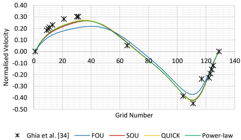
**Fig. 12.** Comparison of velocity field of  $u_y$  at the middle line of the y-axis of the lid-driven cavity at  $Re = 400$
