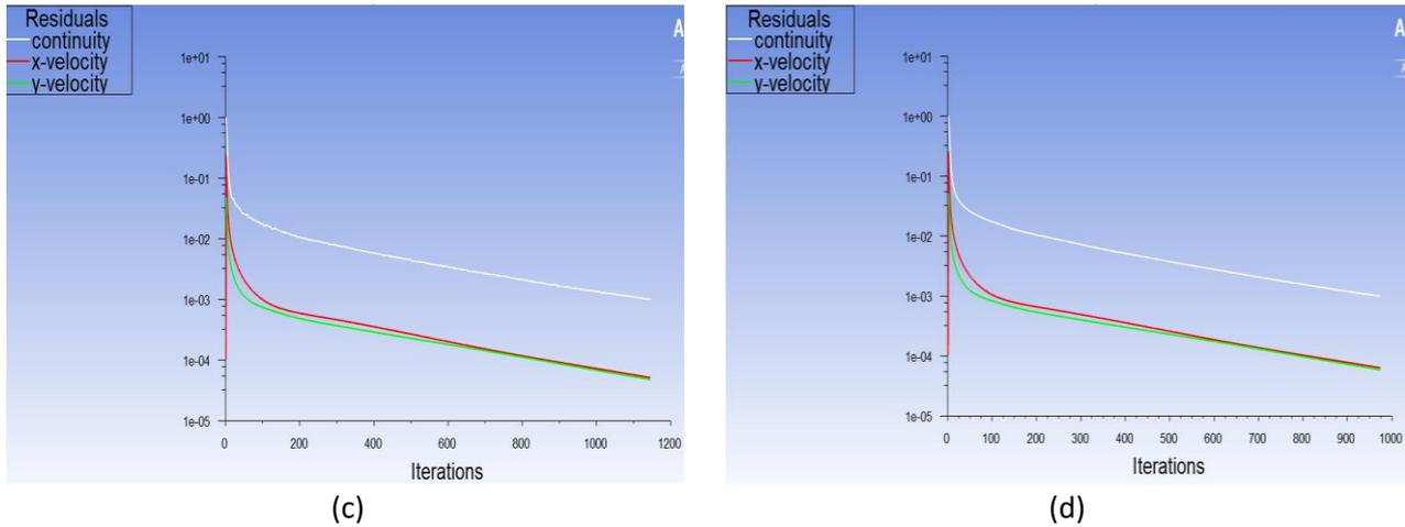
**Fig. 8.** Convergence plot at  $Re = 400$  computed by: (a) FOU; (b) SOU; (c) QUICK; (d) power-law scheme with grid number  $129 \times 129$
