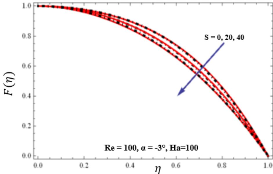
Fig. 5. Velocity variation profile for various  $S$  in converging channel case
