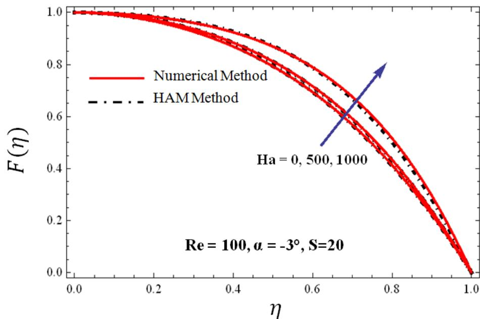
Fig. 2. Velocity profile variation for various Hartmann number (Ha) in converging channel case
