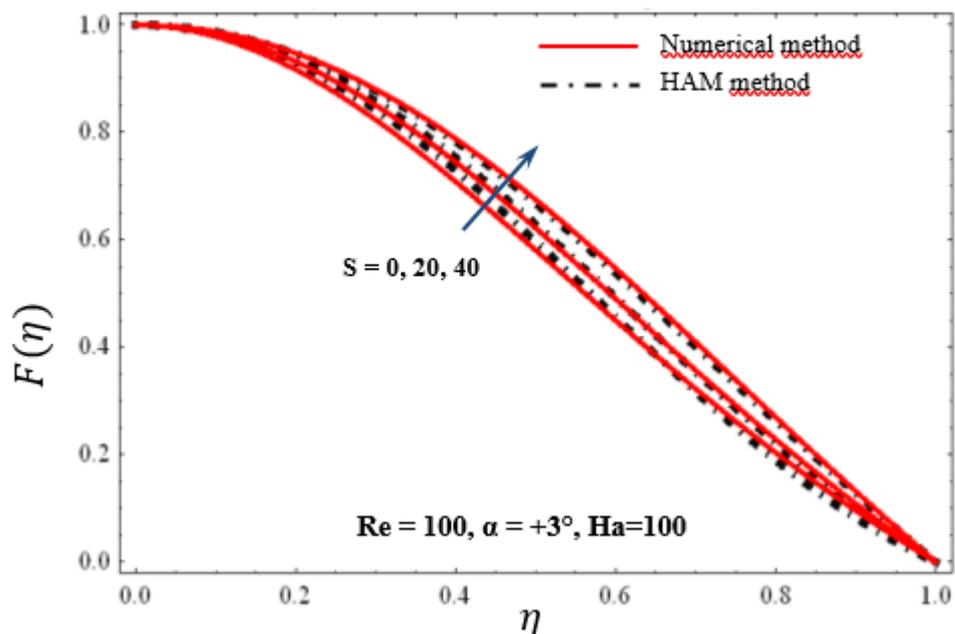
**Fig. 4.** Velocity variation profile for various  $S$  in diverging channel case
