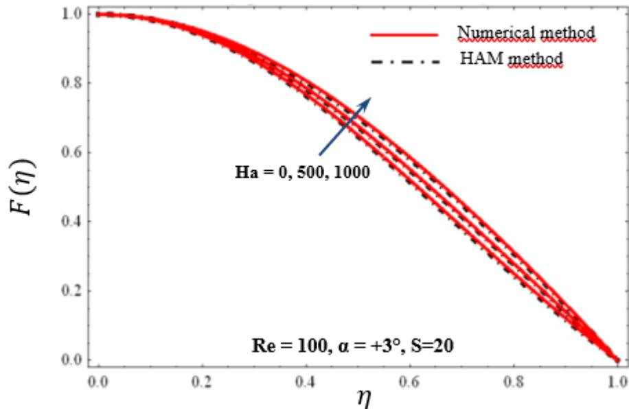
**Fig. 3.** Velocity variation profile for various Hartmann numbers in diverging channel case
