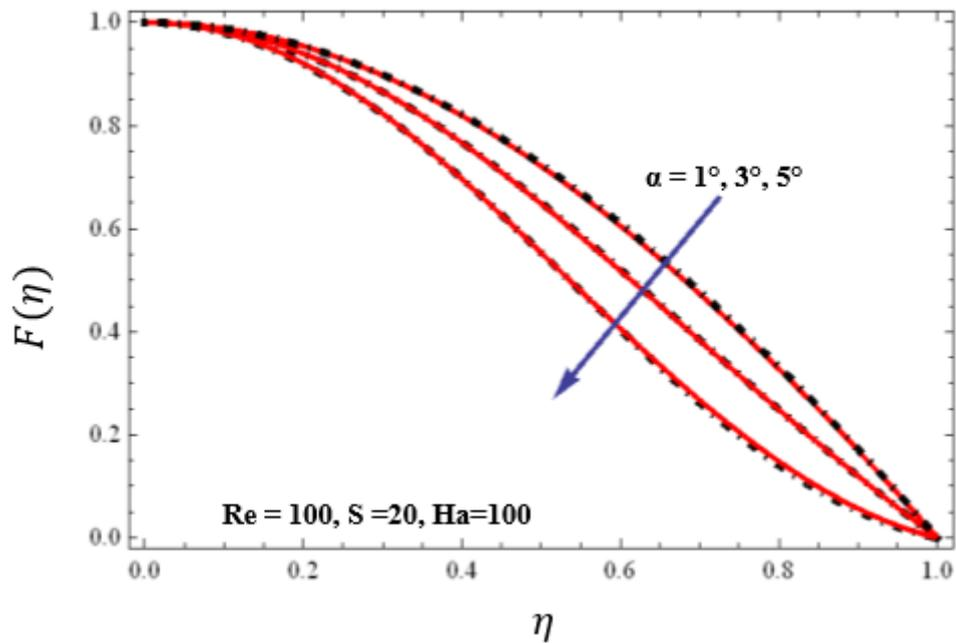
**Fig. 7.** Velocity variation profile for various inclination angles ( $\alpha$ ) in diverging channel case
