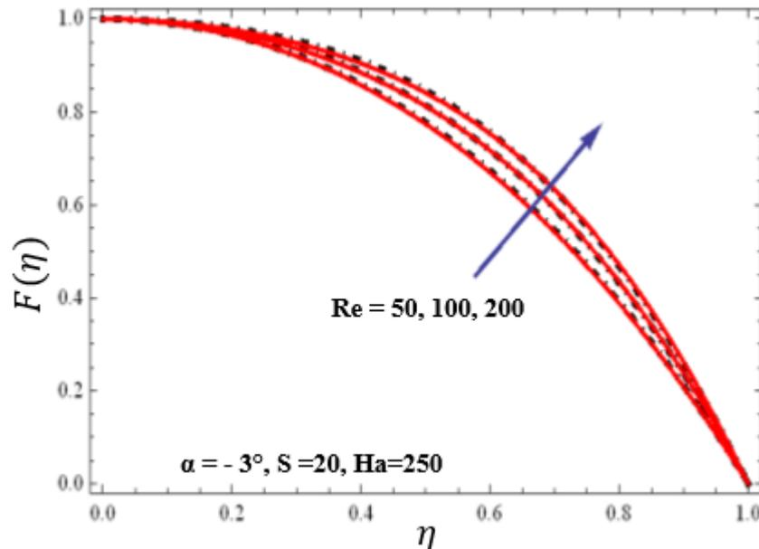
Fig. 9. Velocity variation profile for various Reynolds numbers in converging channel case
