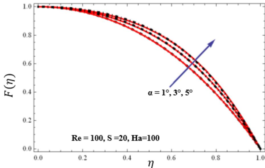
Fig. 6. Velocity variation profile for various inclination angles ( $\alpha$ ) in converging channel case
