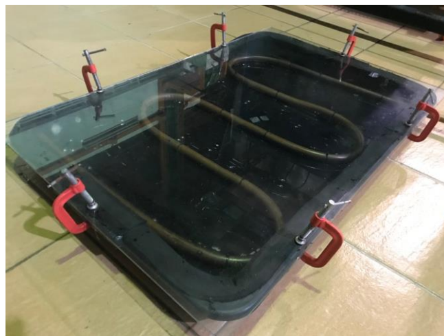
Fig. 1. Absorber collector with glass placed on top
