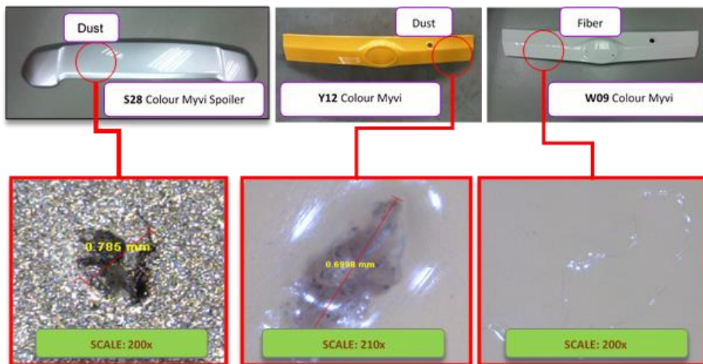
Fig. 2. Sample contamination of dust and fibre in painting line (Source from Combat Coating (M) Sdn Bhd)
