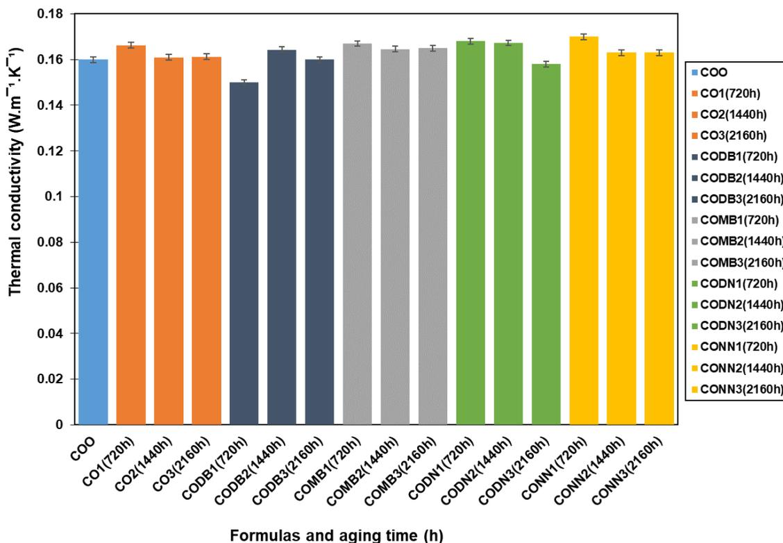
Fig. 5. Thermal conductivity of JCCO aged with or without ceramic balls
