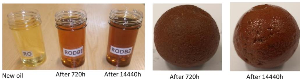
Fig. 12. Aspect of JCRO and ceramic ball before or after heat treatment
