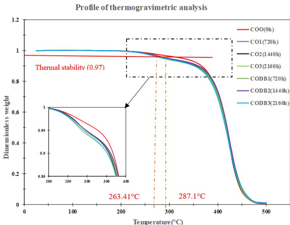
Fig. 8. TGA profile of the different JCCO aged with or without Ceramic balls
