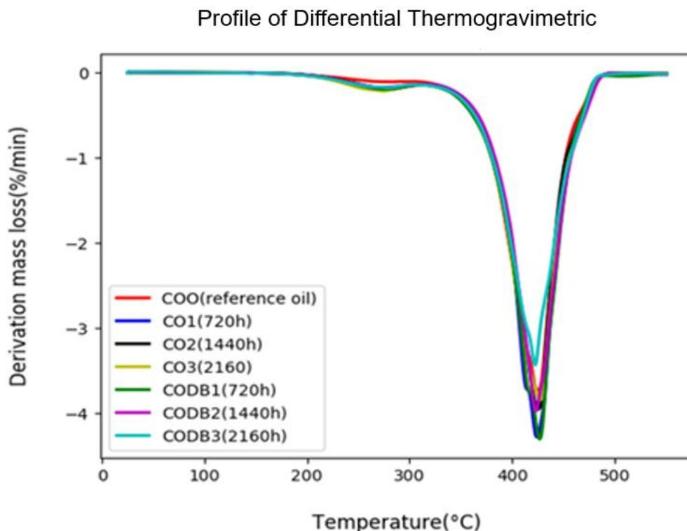
Fig. 7. DTA profile of the different JCCO aged with or without Ceramic balls
