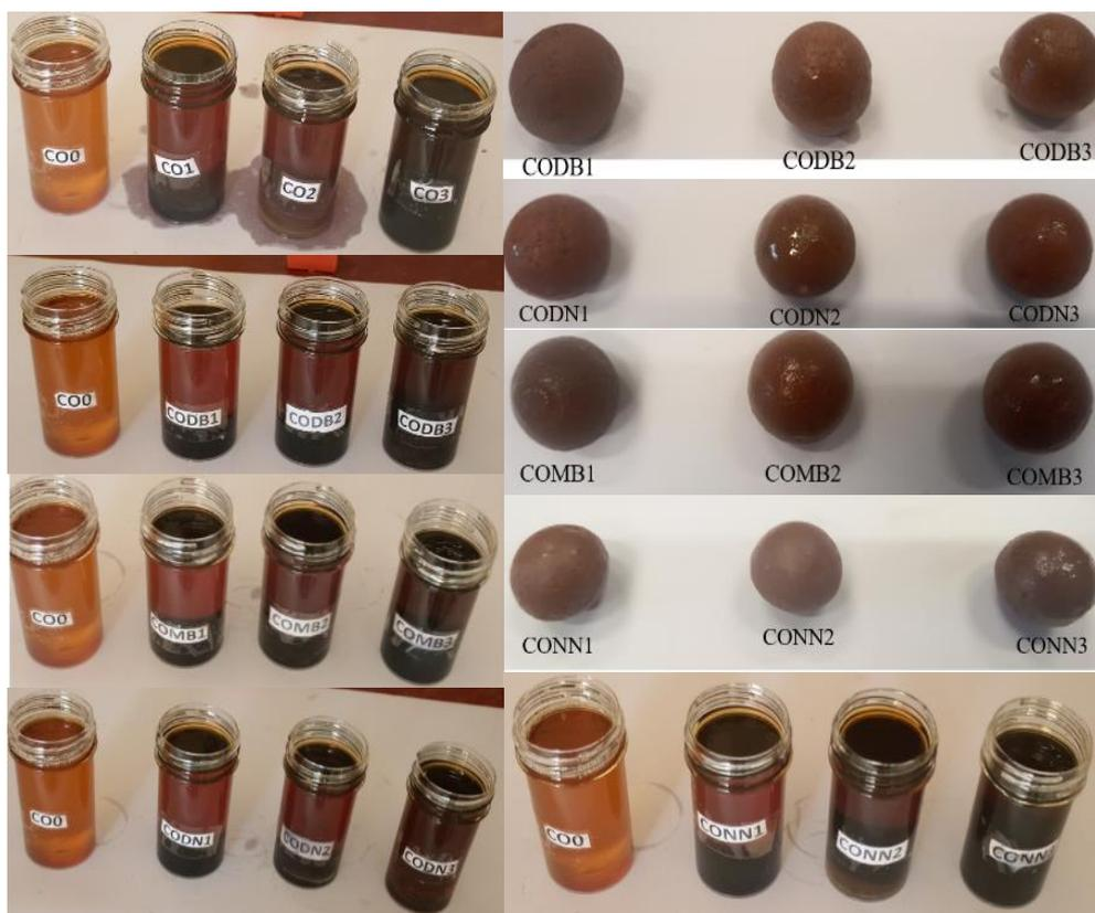
**Fig. 3.** Oil and ceramic balls before or after heat treatment with different sample comparison
