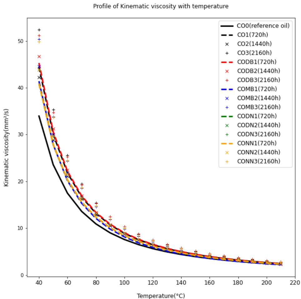
**Fig. 6.** Kinematic viscosity of the oil aged with or without ceramic balls
