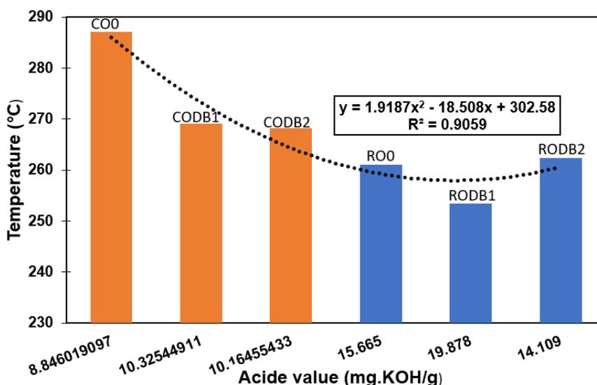
Fig. 10. Thermal stability temperature (°C) of JCCO and JCRO under heat treatment in contact with ceramic balls
