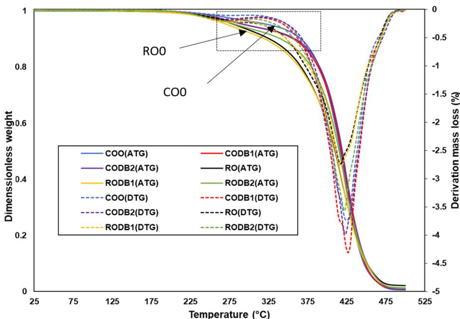
Fig. 9. ATG and DTG profile of JCCO and JCRO in contact with ceramic ball during 1440h
