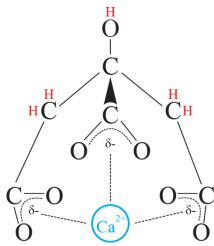
**Fig. 1.** Schematic of citrate ions chelating on calcium ions
