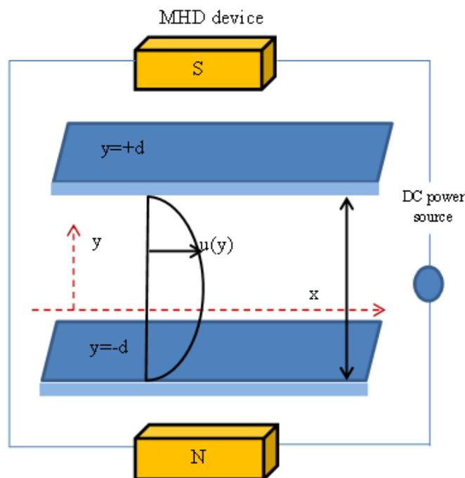
**Fig. 1.** Diagram of the physical system of flow problem
