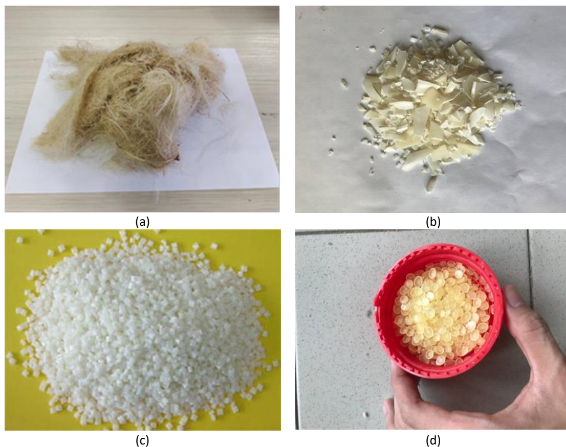
Fig. 1. Materials used in the research: (a) kenaf fibre (b) rHIPS (c) ABS (d) MAPP
