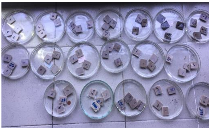
Fig. 3. Water absorption test of rHIPS/ABS/kenaf composite
