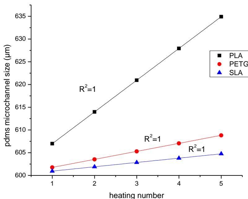
**Fig. 6.** PDMS microchannel size after printed using the 3D printed mold
