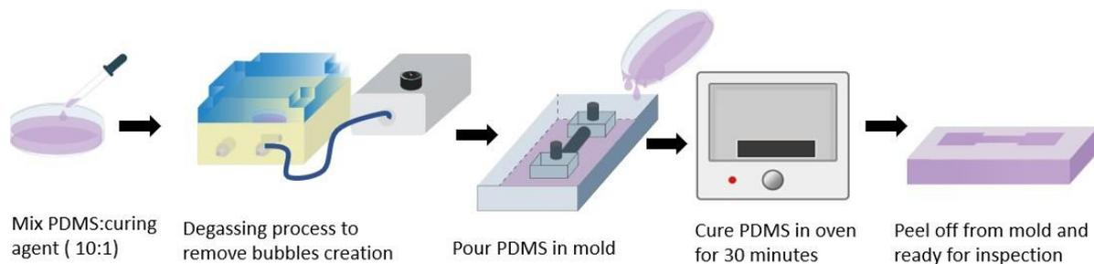
**Fig. 2.** Schematic of PDMS microchannel fabrication process
