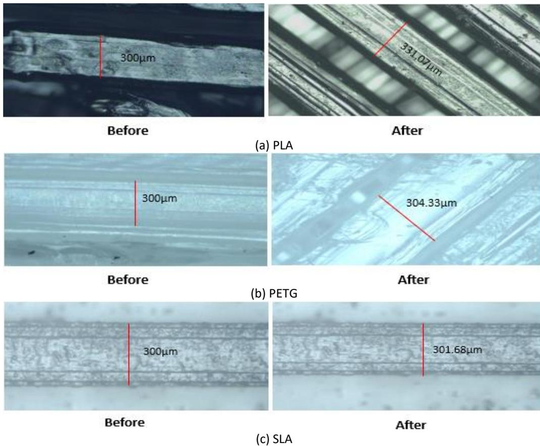
**Fig. 3.** Size of 3D-printer mold structure before and after the pre-heated procedure
