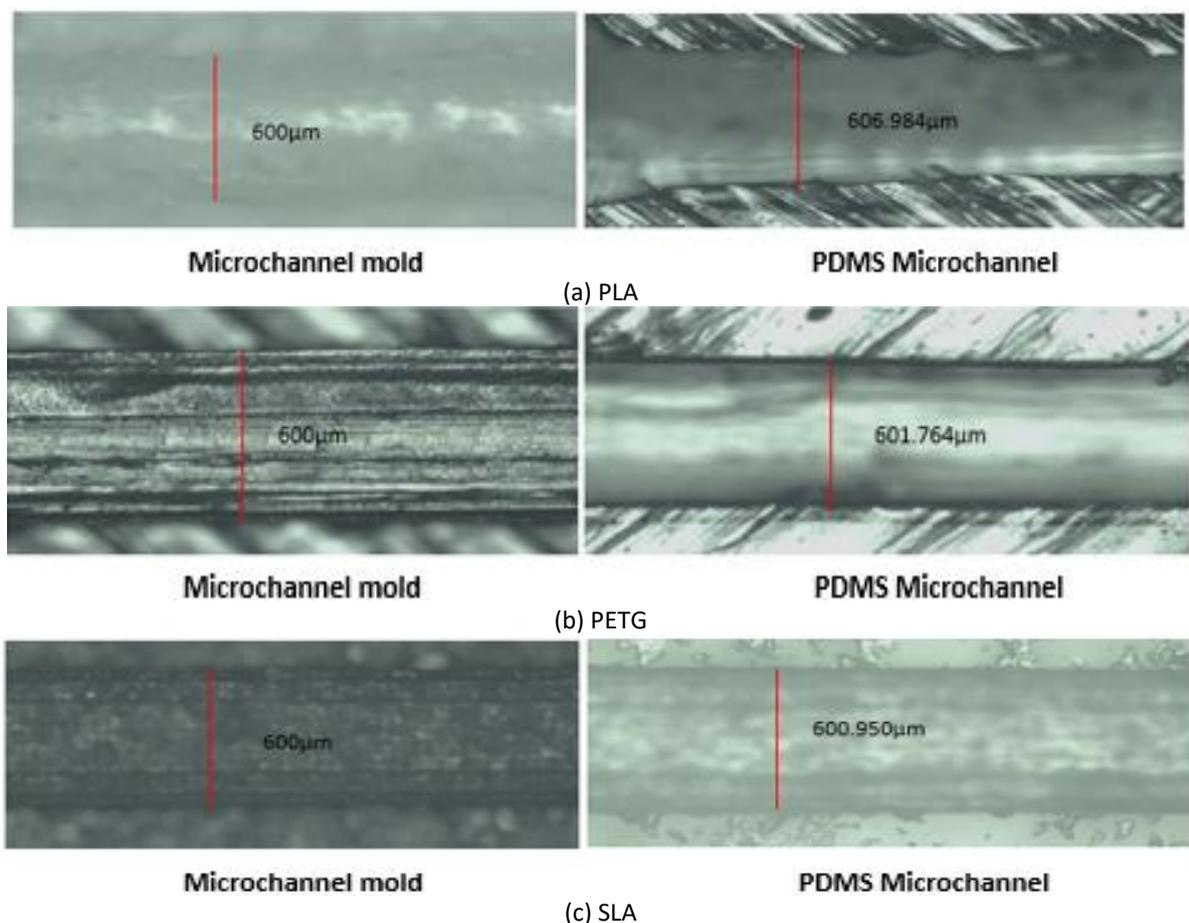
**Fig. 5.** Size of 3D-printer mold and PDMS microchannel printed using the mold
