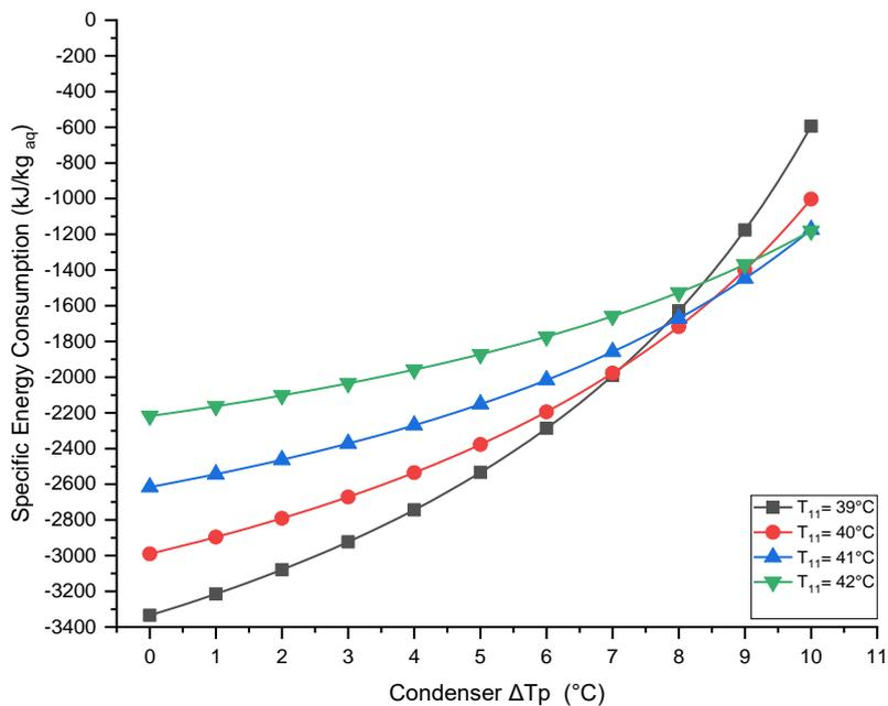
**Fig. 6.** Graph Specific Energy Consumption vs. Pinch Point Difference Condenser power plant at different condenser temperatures
