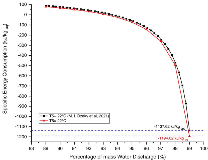
**Fig. 10.** Graph Specific Energy Consumption vs. percentage of mass water discharge previous [24] and currently research
