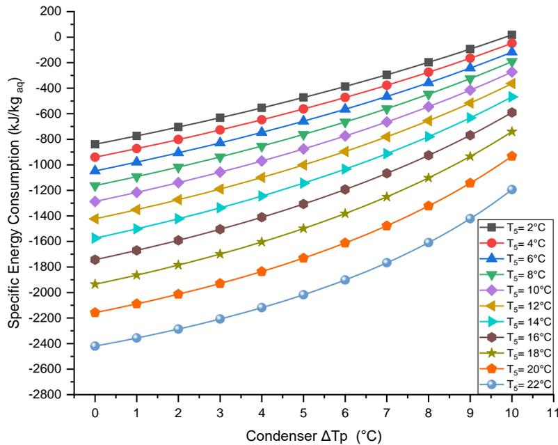
**Fig. 4.** Graph Specific Energy Consumption vs. Pinch Point Difference Condenser power plant at different temperatures in a cyclone separator
