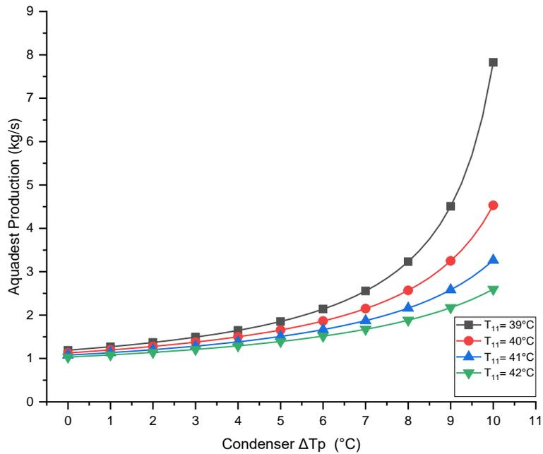
**Fig. 5.** Graph Aquadest Production vs. Pinch Point Difference Condenser power plant at different condenser temperatures
