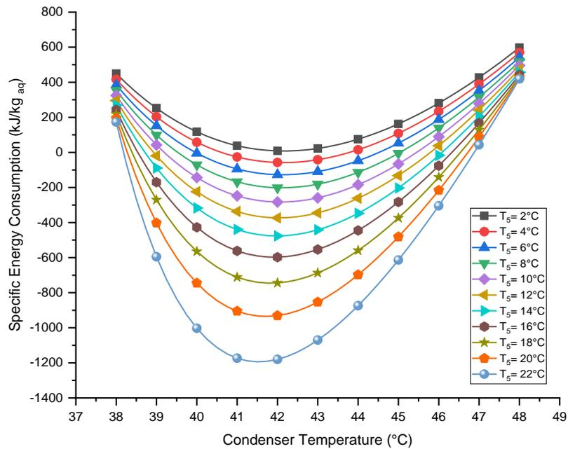
**Fig. 2.** Graph Specific Energy Consumption vs Condenser Temperature at different temperatures in a cyclone separator
