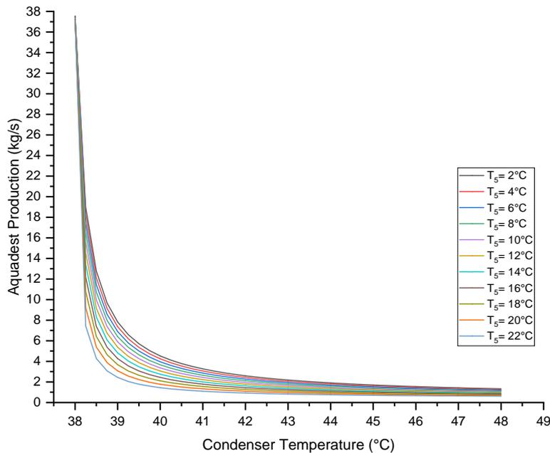
**Fig. 3.** Graph Aquadest Production vs. Condenser Temperature at different temperatures in a cyclone separator
