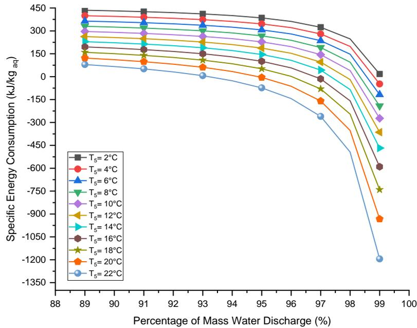
**Fig. 9.** Graph Specific Energy Consumption vs. Percentage of mass water discharge at different temperatures in a cyclone separator
