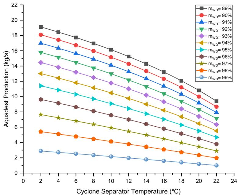
**Fig. 8.** Graph Aquadest Production vs. Temperature in cyclone separator at different percentages of mass water discharge.
