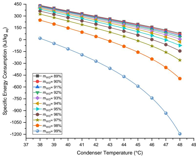
**Fig. 7.** Graph Specific Energy Consumption Vs. Condenser Temperature at the different percentages of mass water discharge
