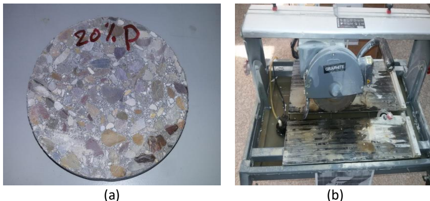
Fig. 3. (a) specimen, (b) concrete cutter
