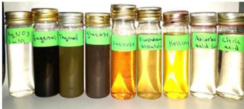
Fig. 2. Control solution ( \text{AgNO}_3 ) and different natural compounds added to \text{AgNO}_3 as reducing agents (from left to right): eugenol, thymol, D-glucose, sucrose, coumarin, scopolamine, kelling, L-ascorbic acid and citric acid
