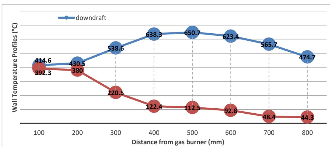
**Fig. 5.** Temperature profile for downdraft and fluidized bed in a combustion chamber
