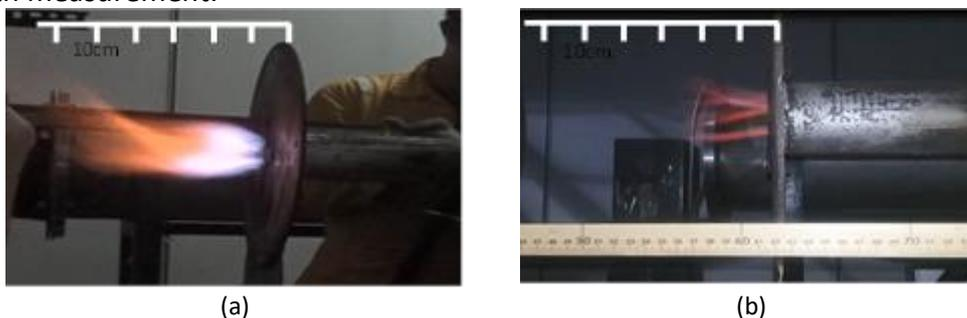
Fig. 7. (a)Downdraft Flame; (b) Fluidized bed Flame
