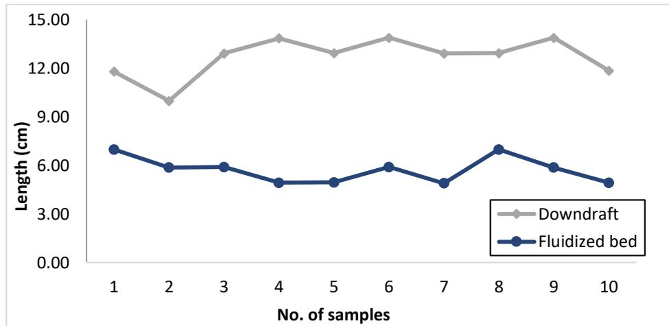
Fig. 6. Flame Length measurement for downdraft and fluidized bed gasifier
