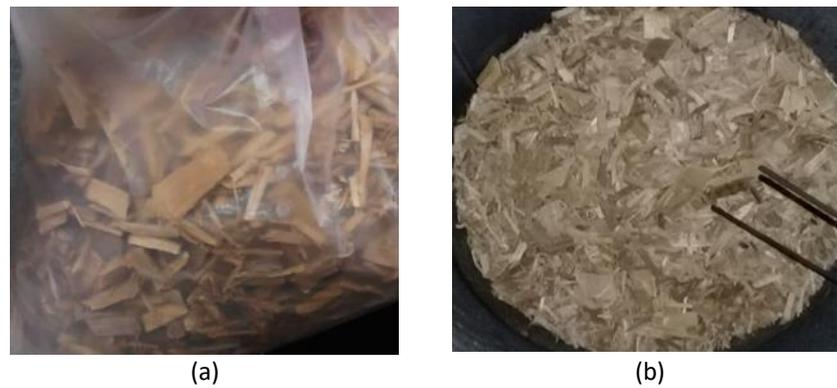
**Fig. 1.** (a)Downdraft Feedstock; (b) Fluidized Bed Feedstock
