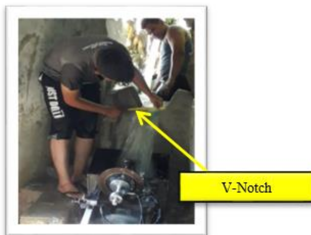
Fig. 2. Measurement of v-notch weir dimensions
