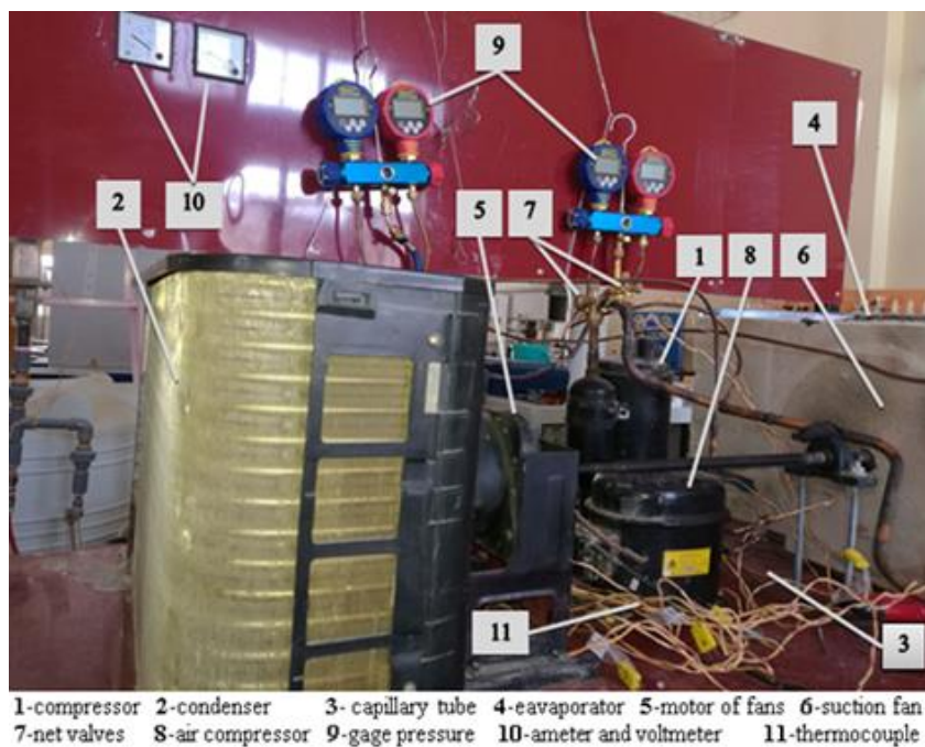
Fig. 2. The experimental system of the air conditioner
