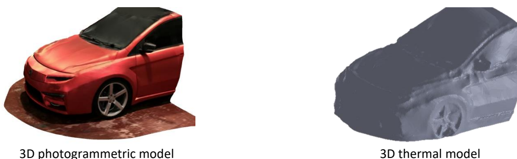
Fig. 8. Development of 3D model for thermal analysis using photogrammetry
