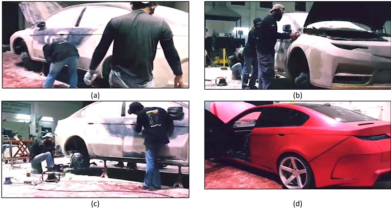
Fig. 6. Car body panels modifications: (a) polyurethane (PU) foam spraying process, (b) sanding process (c) cementing process and (d) vinyl wrapping process
