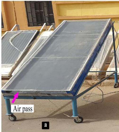
Length: 2 m . Width: 1 m. Thickness: 0.08 m/0.16 m. Absorber: plat aluminum painted in black+ the sand dunes. Insulation: polystyrene. Angle of orientation: 32°
