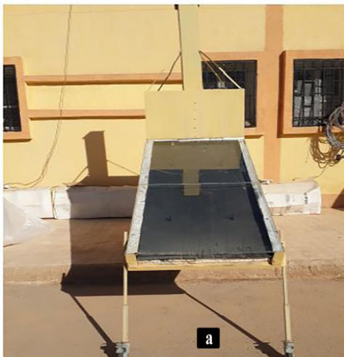
Length of collector: 2 m. Width: 1 m. Thickness: 0.055 m Depth of chamber: 0.7 m Length of chamber: 0.87 m. Width of chamber: 0.68. Absorber: plate aluminum. Insulation: Polystyrene. Angle of orientation: 31°
