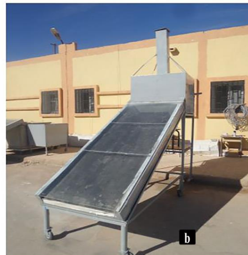
Length of collector: 2.53 m. Width: 1 m. Thickness: 0.13 m 1st passage: 0.065 m. 2nd passage: 0.065 m. Depth of chamber: 0.7 m Length of chamber: 0.87 m. Width of chamber: 0.68. Absorber: plate aluminum. Insulation: Polystyrene. Angle of orientation: 32°
