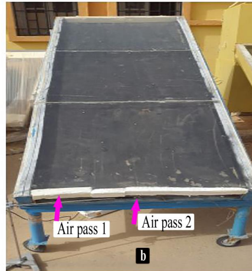
Length: 2 m . Width: 1 m. Thickness: 0.13 m. 1st passage:0.065 m. 2nd passage:0.065 m. absorber: plate aluminum. Insulation: Glass wool. Orientation angle: 32°
