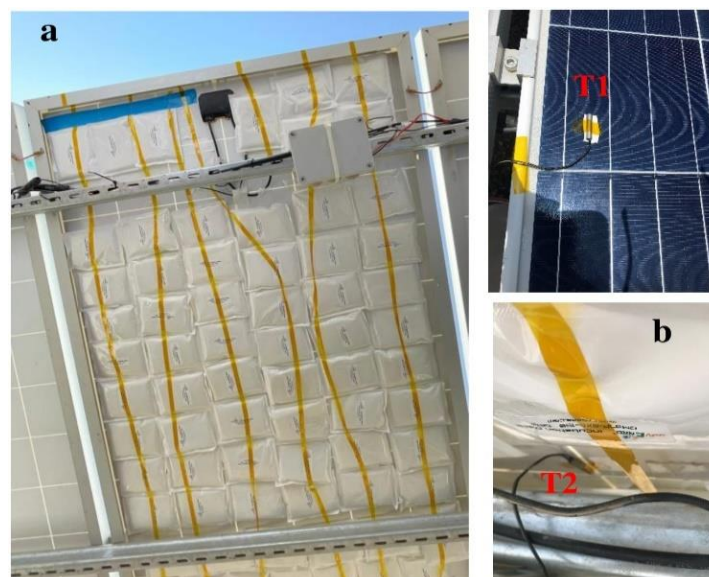
Fig. 4. (a) There are PCM collections with PCM-OM37P content, (b) the positions of both thermocouples rear and front
