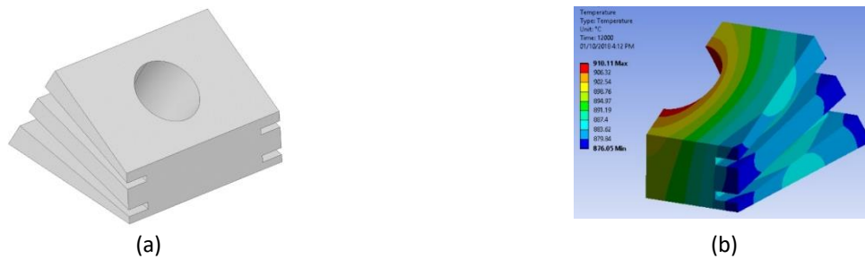
Fig. 3. CAD model of 3-fins design [13] and (b) Temperature distribution in 3-fins model, at maximum engine speed
