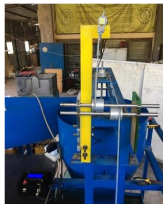
Fig. 2. Low-speed water canal (a) Side view, (b) Top view, and (c) Prony brake system [17]
