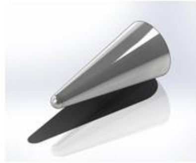
Fig. 1. Spherical blunted conic nose and profile with parameters [10]
