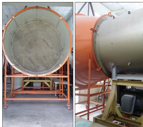
Fig. 1. Universiti Putra Malaysia open-loop wind tunnel specification [20]
