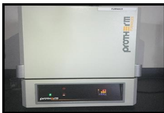
Fig. 3. Electric furnace for fire resistance test
