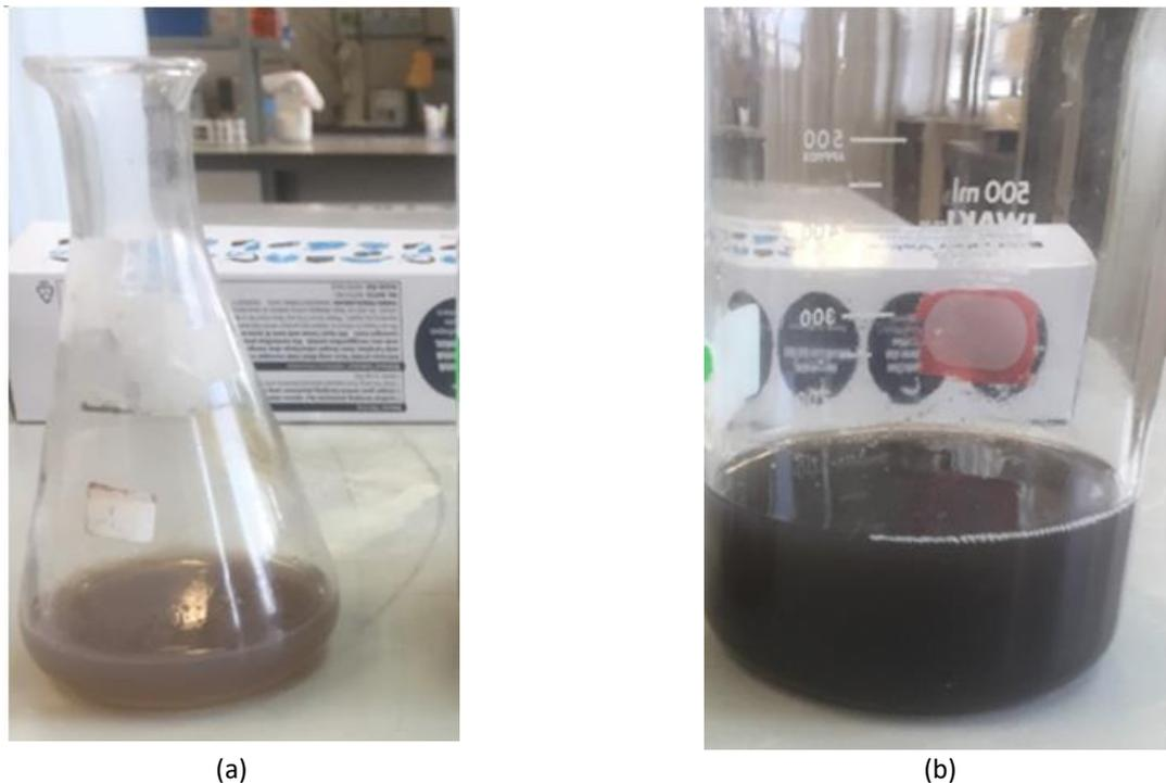
**Fig. 4.** (a) wastewater after adsorption process at 180 min contact time and (b) wastewater before undergoes any adsorption process
