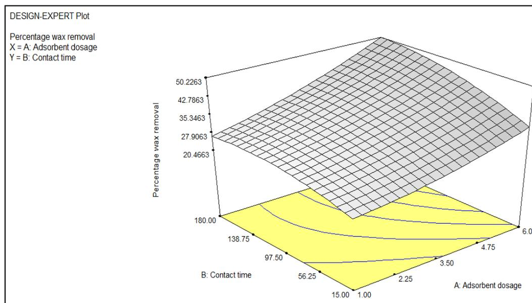
**Fig. 2.** Effect of CNCs dosage and contact time to the percentage of wax removal
