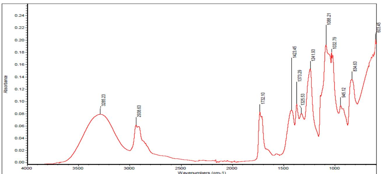
Fig. 1. FTIR spectra corresponding to 6 %w/v of CNCs/PVA composite
