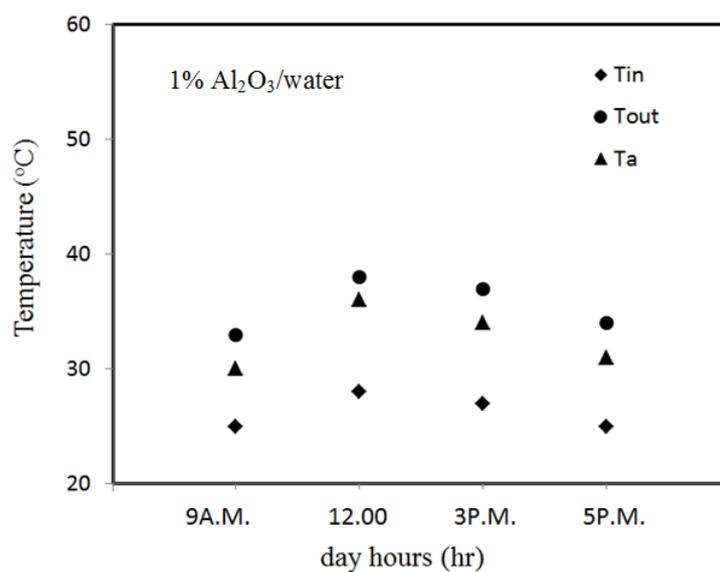
**Fig. 7.** Temperature at inlet, outlet and ambient along the day hours (21/May/2017)
