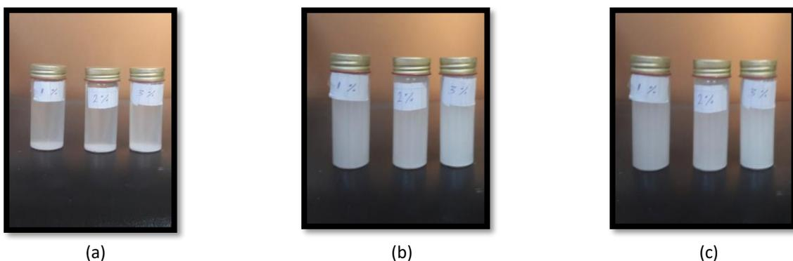
**Fig. 1.** Samples of nanofluid (a) after preparation, (b) after 2 hours and (c) after 4 hours
