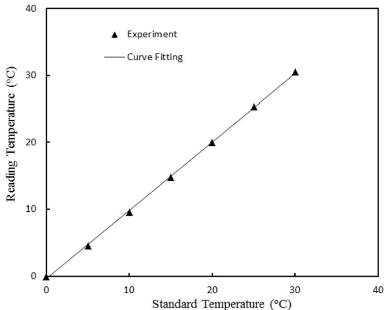
Fig. 3. Calibration data of thermocouples
