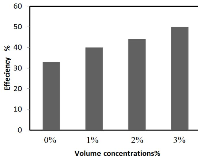
**Fig. 9.** The effect of nanofluid volume concentrations on solar collector efficiency
