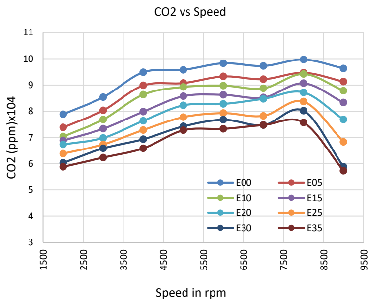
Fig. 11. Effect of Ethanol-gasoline blend on CO emissions using Twin Spark Plug
