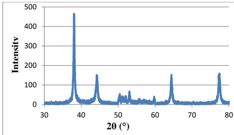
**Fig. 5.** XRD spectra of synthesized AgNPs
