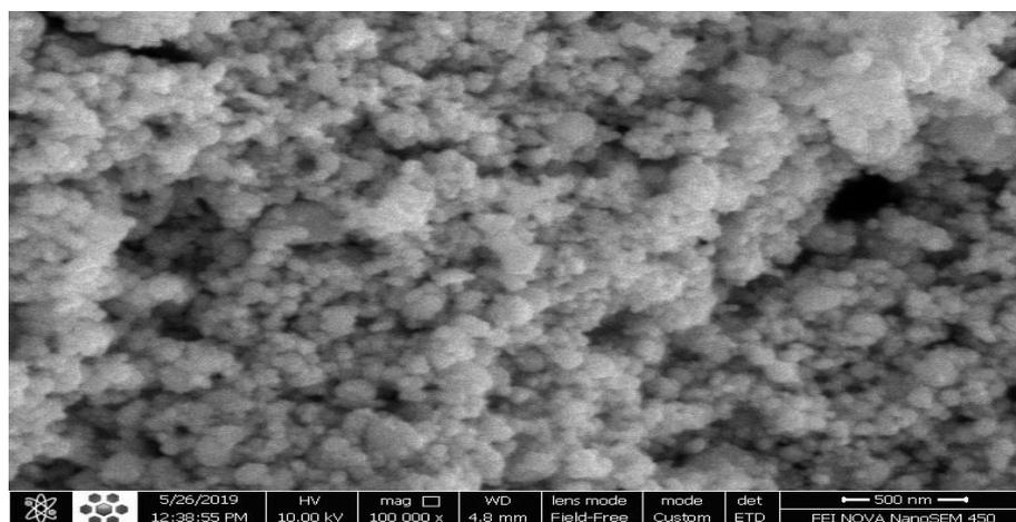
Fig. 3. Surface morphology of synthesized AgNPs in SEM
