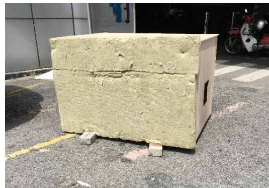
Fig. 9. Test room insulated with Rockwool
