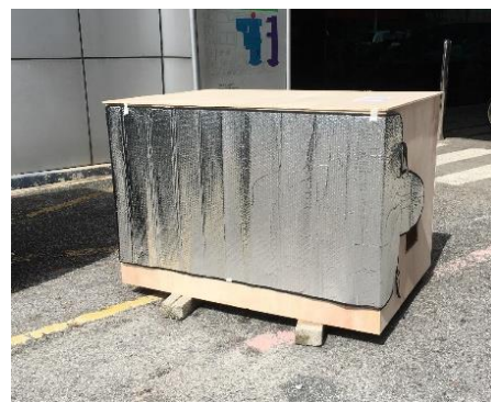
Fig. 7. Test room insulated with PASB
