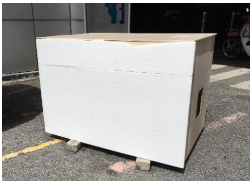
Fig. 8. Test room insulated with EPS board
