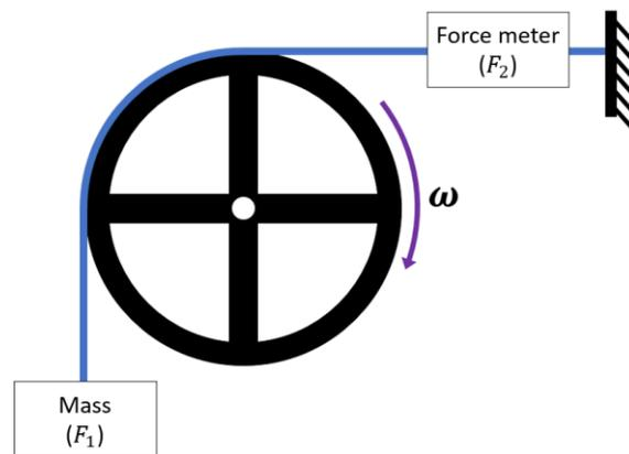
**Fig. 2.** Schematic of prony break
