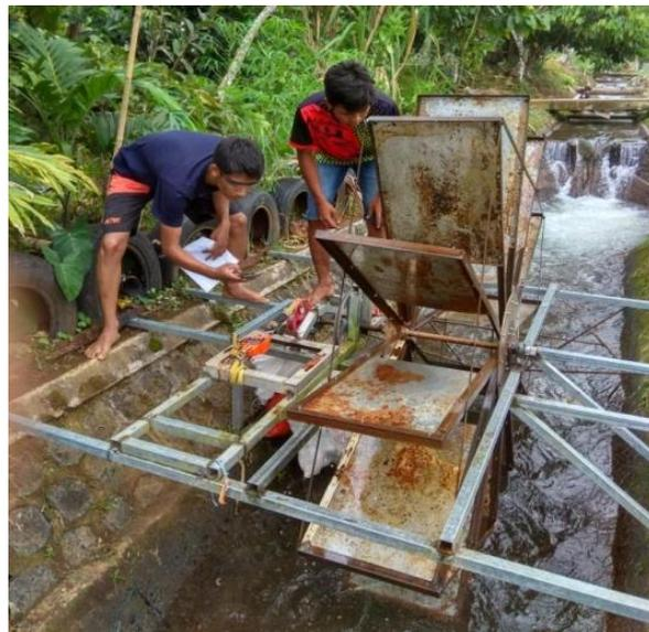
Fig. 5. Undershot waterwheel testing in irrigation
