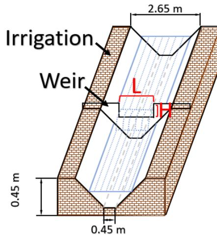
**Fig. 3.** Schematic of rectangular weir
