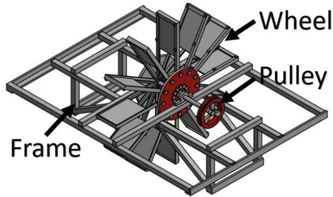
**Fig. 1.** Schematic of the undershot waterwheel
