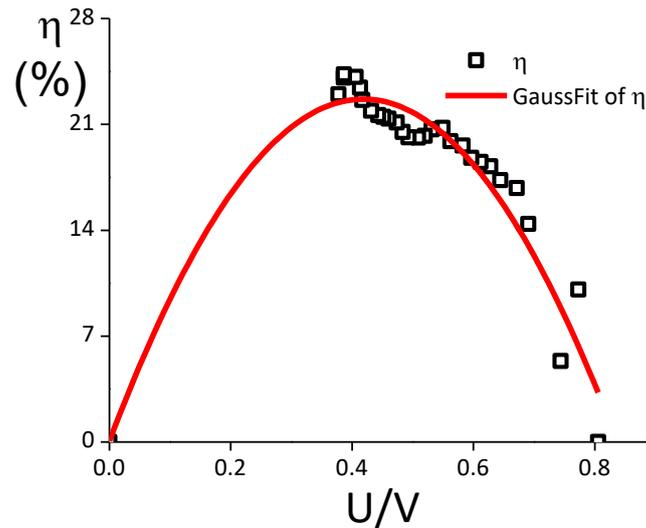
Fig. 4. Undershot waterwheel's mechanics efficiency
