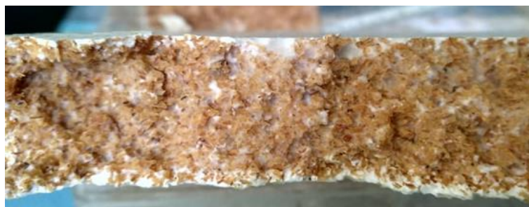
Fig. 8. A cross section of the mycelium-based composite board
