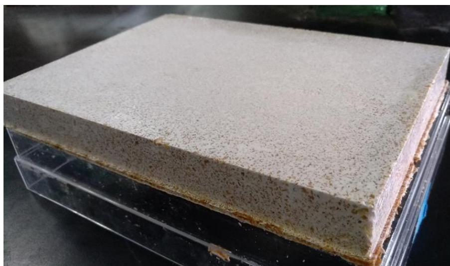
Fig. 2. Self-assembly bio-composite from RWS inoculated with mycelium before hot press
