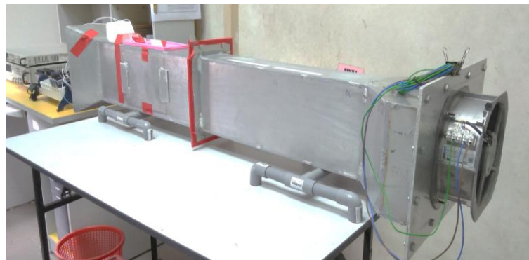
Fig. 2. Completed (a) battery module and (b) air tunnel
