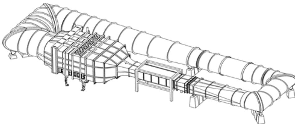
**Fig. 1.** Schematic layout of Universiti Teknologi Malaysia's wind tunnel
