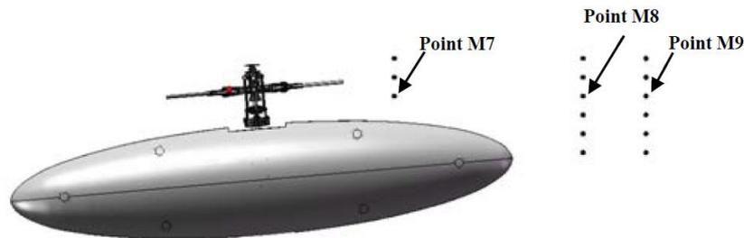
**Fig. 11.** Point designations for No Pylon Configuration
