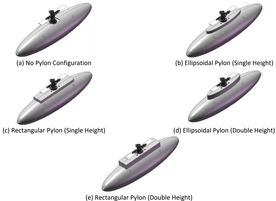
**Fig. 5.** Pylon configurations
