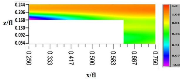
**Fig. 10.** Distribution of  $C_{p0}$  for Rectangular Pylon (Double Height)
