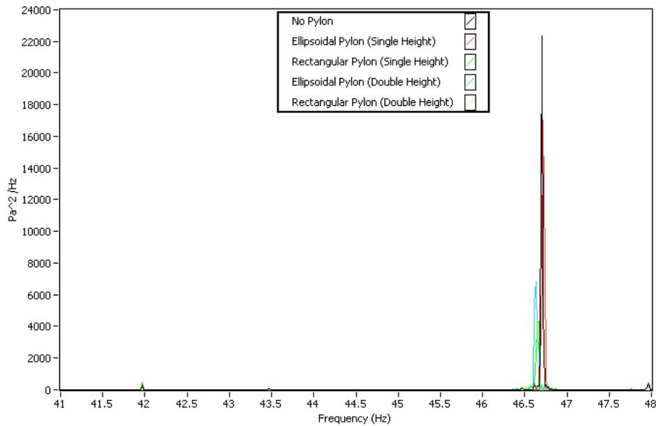
**Fig. 15.** PSD analysis for point M7 at different pylon configurations
