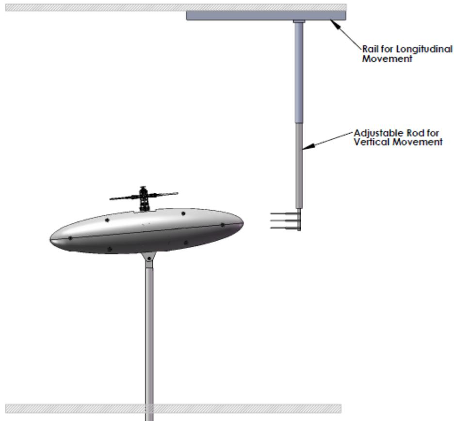
**Fig. 6.** Schematic diagram of pressure mapping
