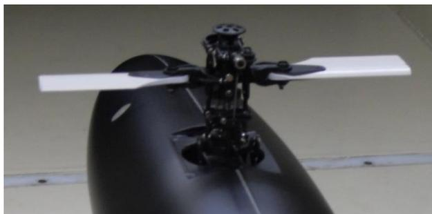
**Fig. 2.** Blade-stubs configuration with single main rotor design
