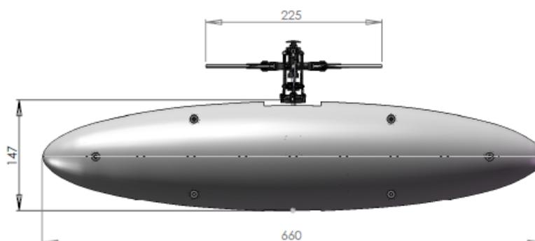
**Fig. 3.** Schematic drawing of the model (dimension in mm)
