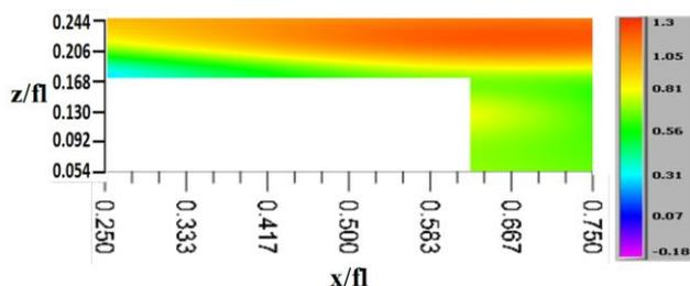
**Fig. 9.** Distribution of  $C_{p_0}$  for Ellipsoidal Pylon (Double Height)
