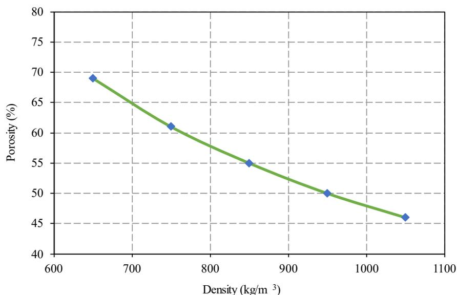
**Fig. 10.** Porosity of lightweight foamed concrete of different densities
