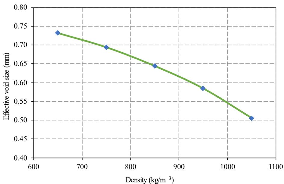
**Fig. 9.** Effective void size of lightweight foamed concrete of different densities
