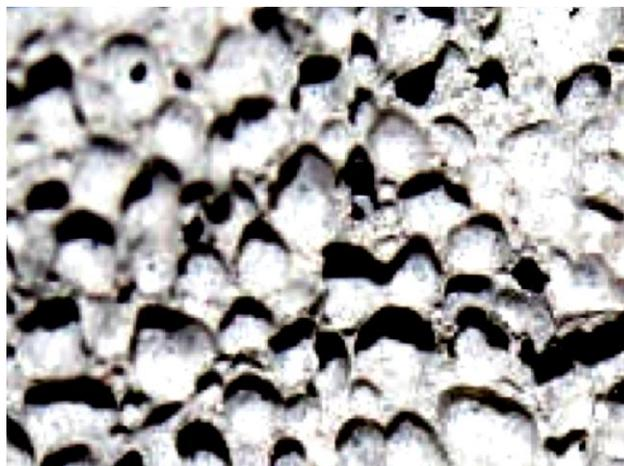
**Fig. 7.** Void size and distribution of lightweight foamed concrete of 650 kg/m<sup>3</sup> density
