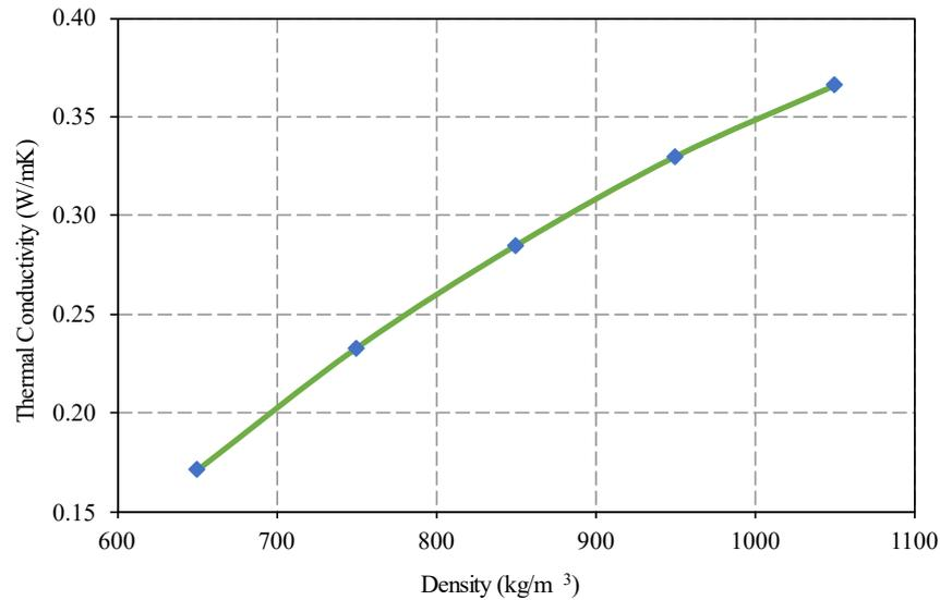
**Fig. 6.** Thermal conductivity of foamed concrete of different densities
