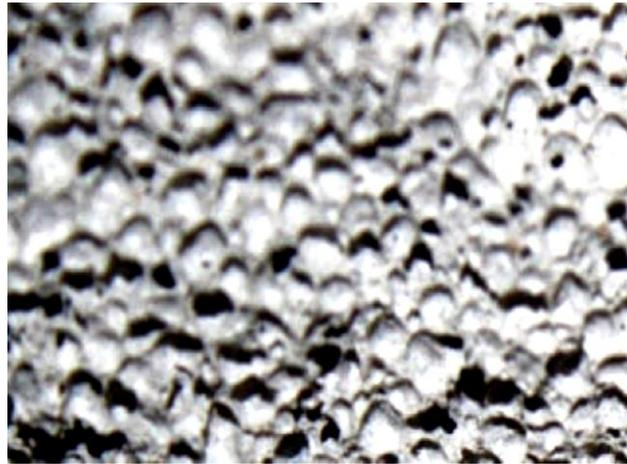
**Fig. 8.** Void size and distribution of lightweight foamed concrete of 1050 kg/m<sup>3</sup> density
