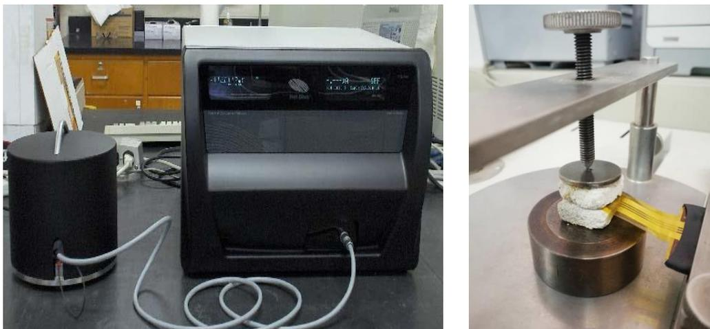
**Fig. 4.** Hot disk thermal constants analyzer apparatus
