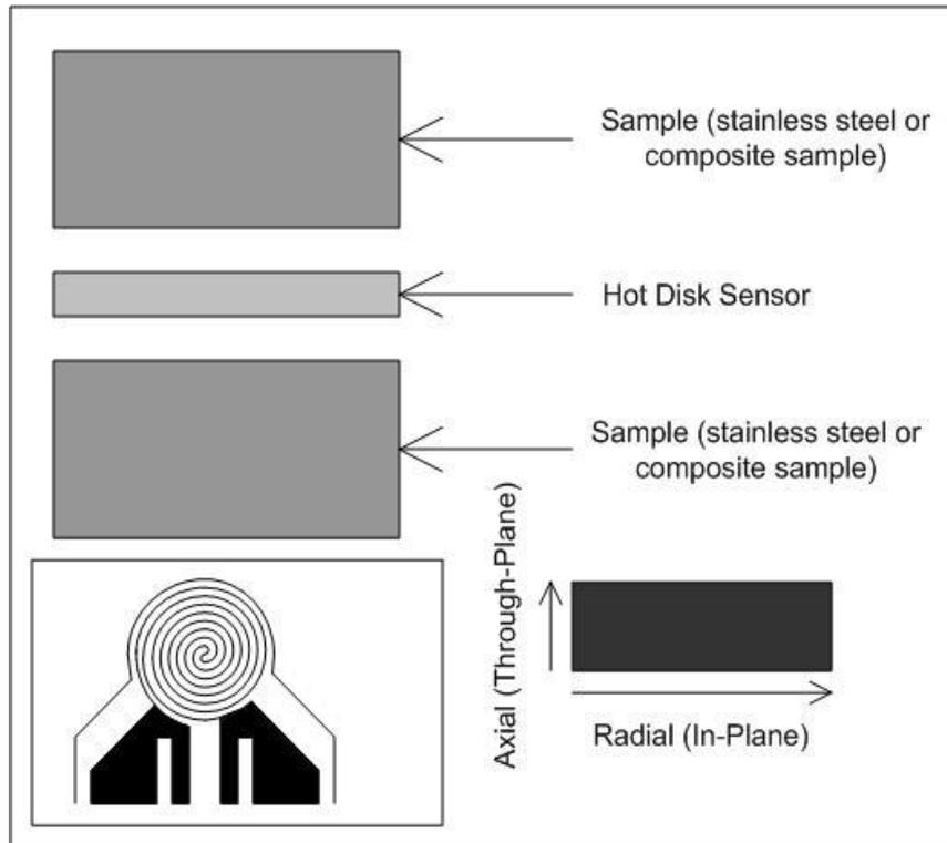
**Fig. 5.** Schematic of samples and sensor for the hot disk the insert at the lower left shows the double spiral heating element
