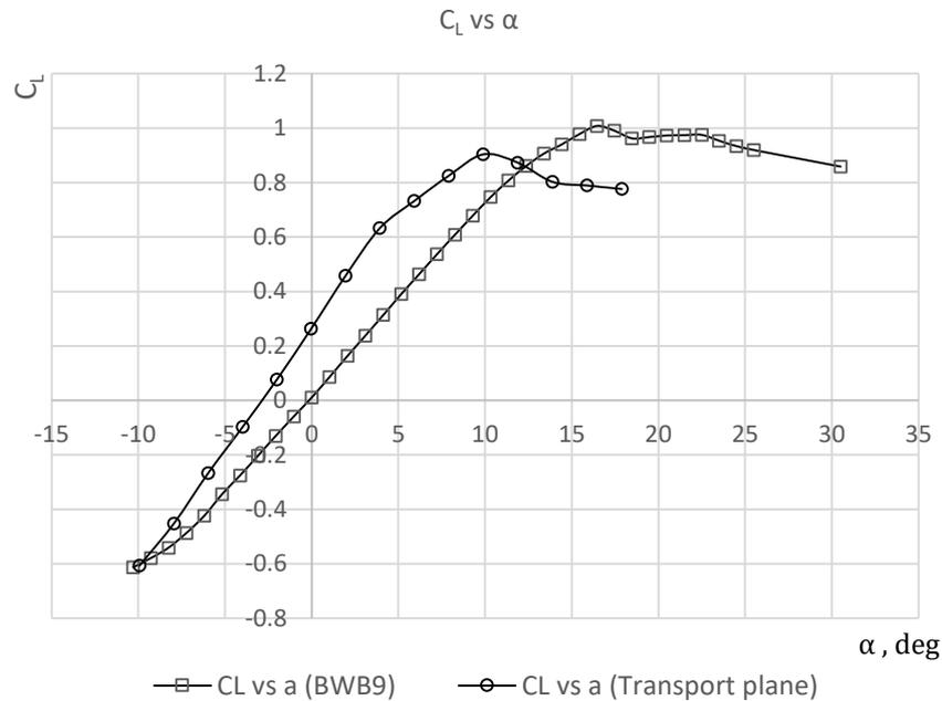
**Fig. 10.** Lift coefficient (CL) versus angle of attack ( $\alpha$ )
