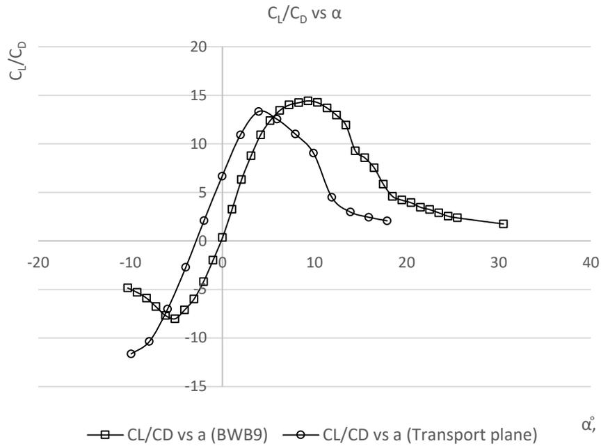
**Fig. 13.** Lift to drag ratio ( $C_L/C_D$ ) versus angle of attack ( $\alpha$ )
