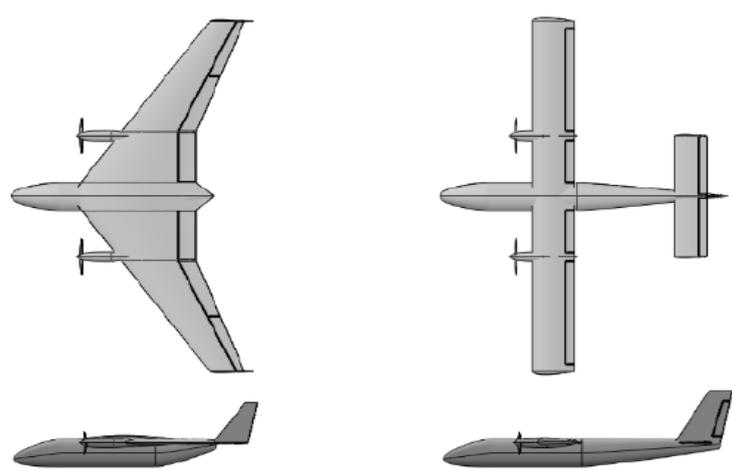
**Fig. 17.** Recommended improvement to BWB Baseline-IX (left) to mimic typical transport aircraft fuselage
