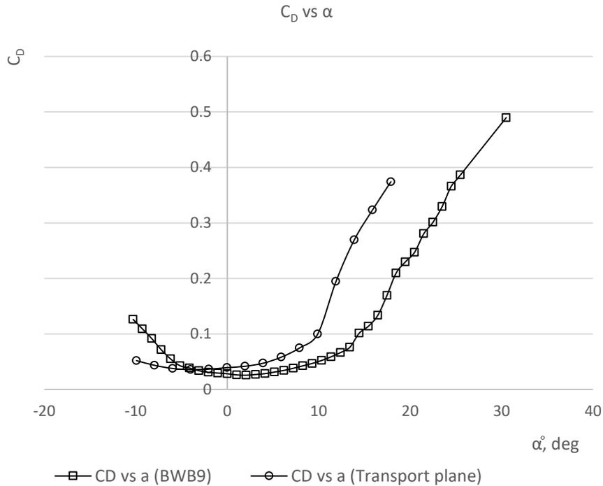
**Fig. 11.** Drag coefficient ( $C_D$ ) versus angle of attack ( $\alpha$ )
