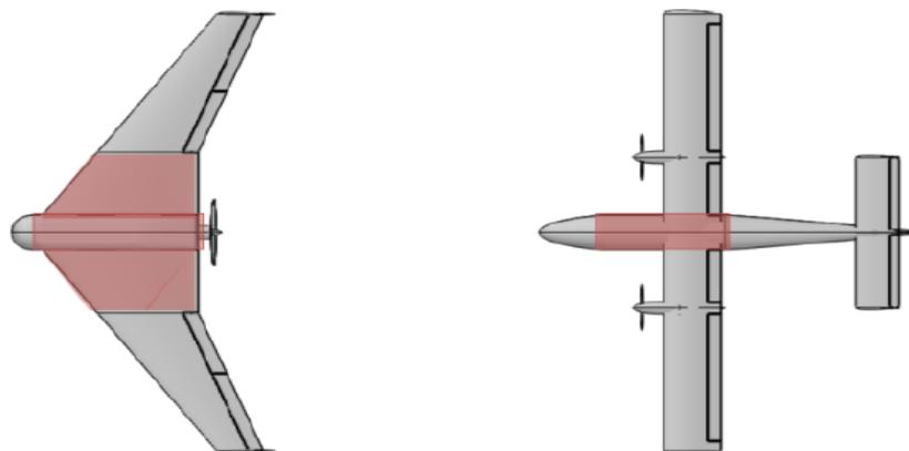
**Fig. 6.** BWB Baseline-IX usable area (left) compared to DHC-6 Twin Otter transport aircraft usable area (right), shaded in red
