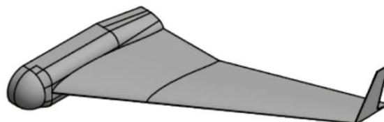
**Fig. 2.** Baseline-IX BWB half model of 1:30 scale for the purpose of printing wind tunnel model
