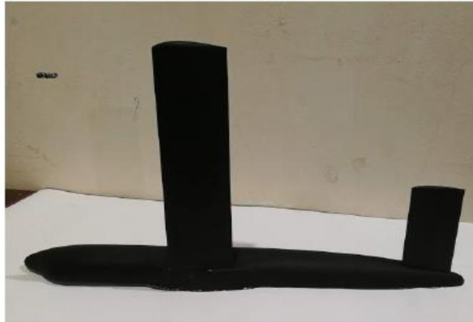
**Fig. 9.** Transport Airplane Twin Otter wind tunnel model
