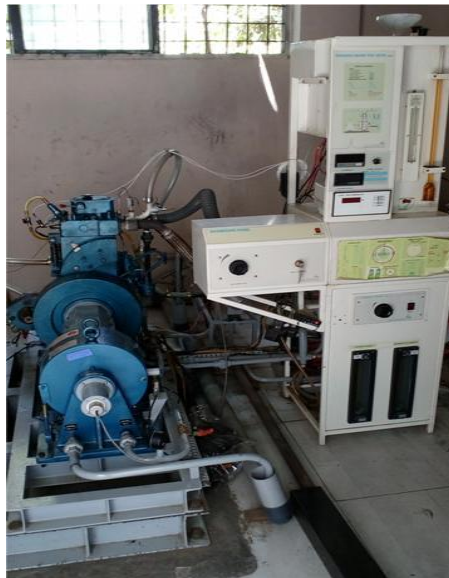
Fig. 1. Computerized S.I engine test rig with exhaust gas analyzer
