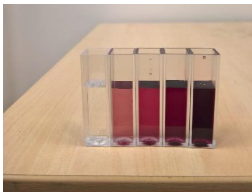
Fig. 1. Picture of the samples with different copper concentrations in 40 wt.% LiBr-H 2 O
