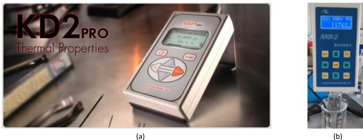
Fig. 1. Measurements equipment; (a) Thermal conductivity equipment (b) Viscosity equipment
