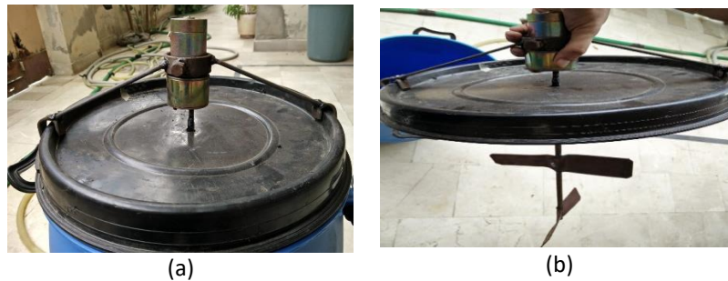
Fig. 15. Flocculation tank (a) gear motor for continuous stirring at 60 RPM (b) Impellers at an angle
