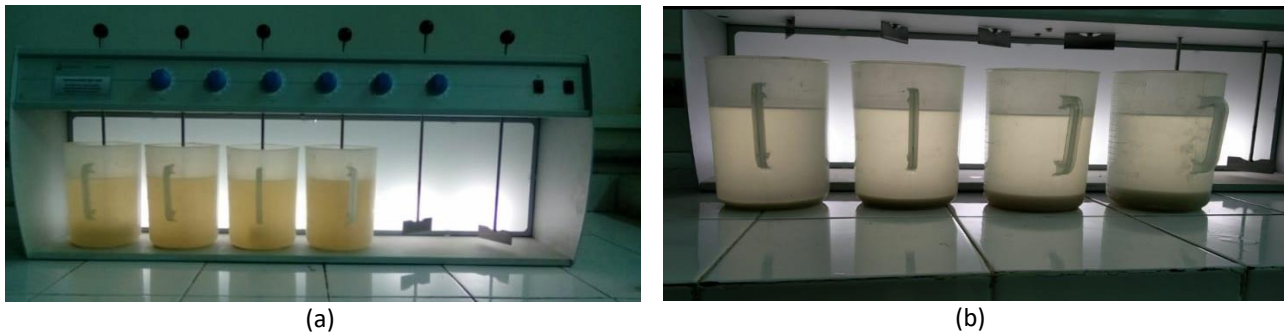
Fig. 10. Coagulant Dosage (a) Samples being tested with various dosage of coagulant, (b) Effects of different coagulant dosage with time
