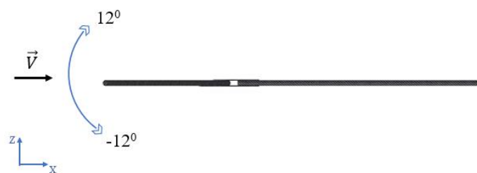
Fig. 3. Angles of tri-copter's frame are investigated
