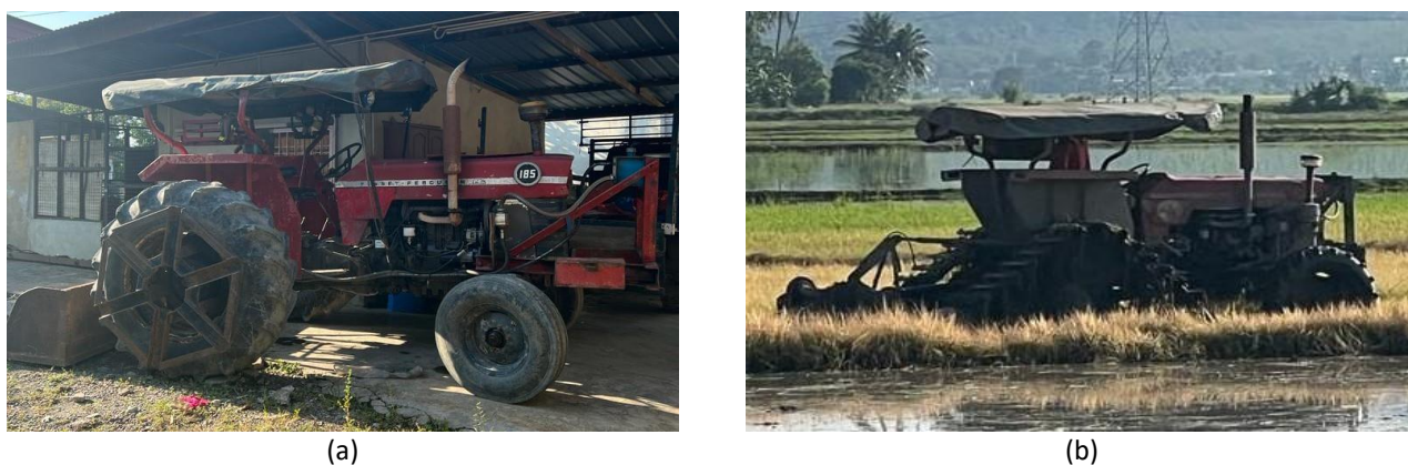
Fig. 5. (a) Rubber-wheeled and (b) Steel half-tracked tractors
