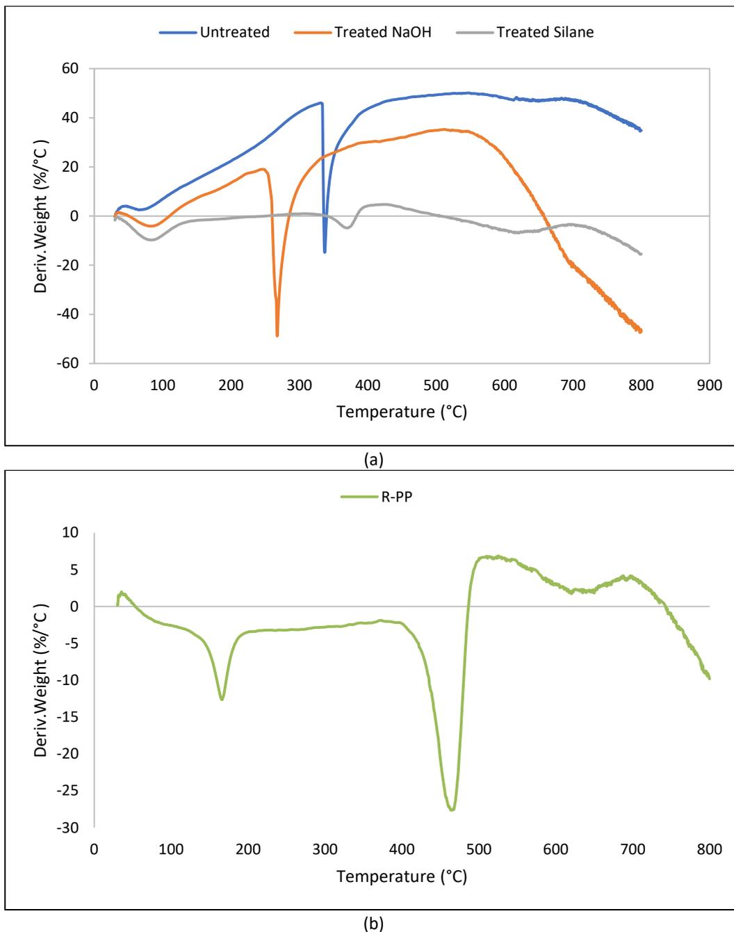
**Fig. 3.** DSC graph of (a) NaOH treated, silane treated, and untreated wood dust and (b) Recycle PP
