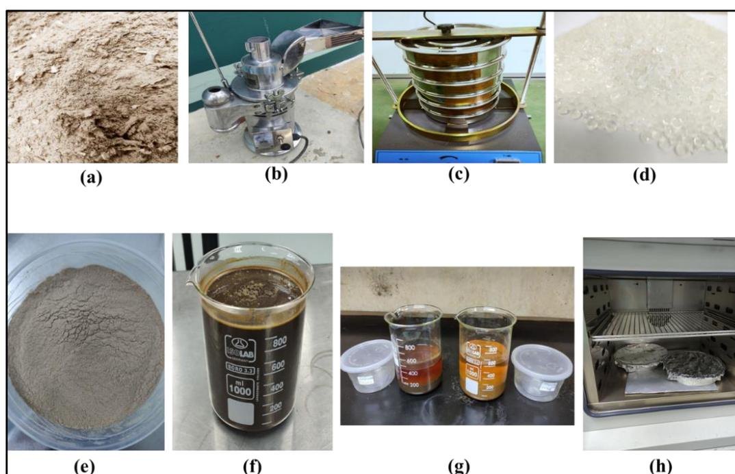
**Fig. 1.** (a) Raw wood dust fibre from the workshop (b) grinder machine for grind into dust (c) Industrial sieve for getting result 125 µm (d) recycled PP pallet form (e) the result of 125 µm wood dust fibre (f) NaOH treatment represent (g) NaOH-Silane and Silane Treatment (h) material after treatment dry on the oven
