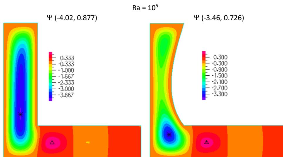
**Fig. 2.** Comparison of the streamlines between rigid and flexible wall models inside L-shaped cavity for various Rayleigh numbers ( $Pr = 0.7, E = 10^9$ )
