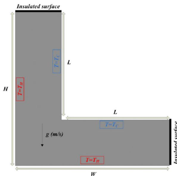
**Fig. 1.** Schematic of the problem under investigation and boundary conditions
