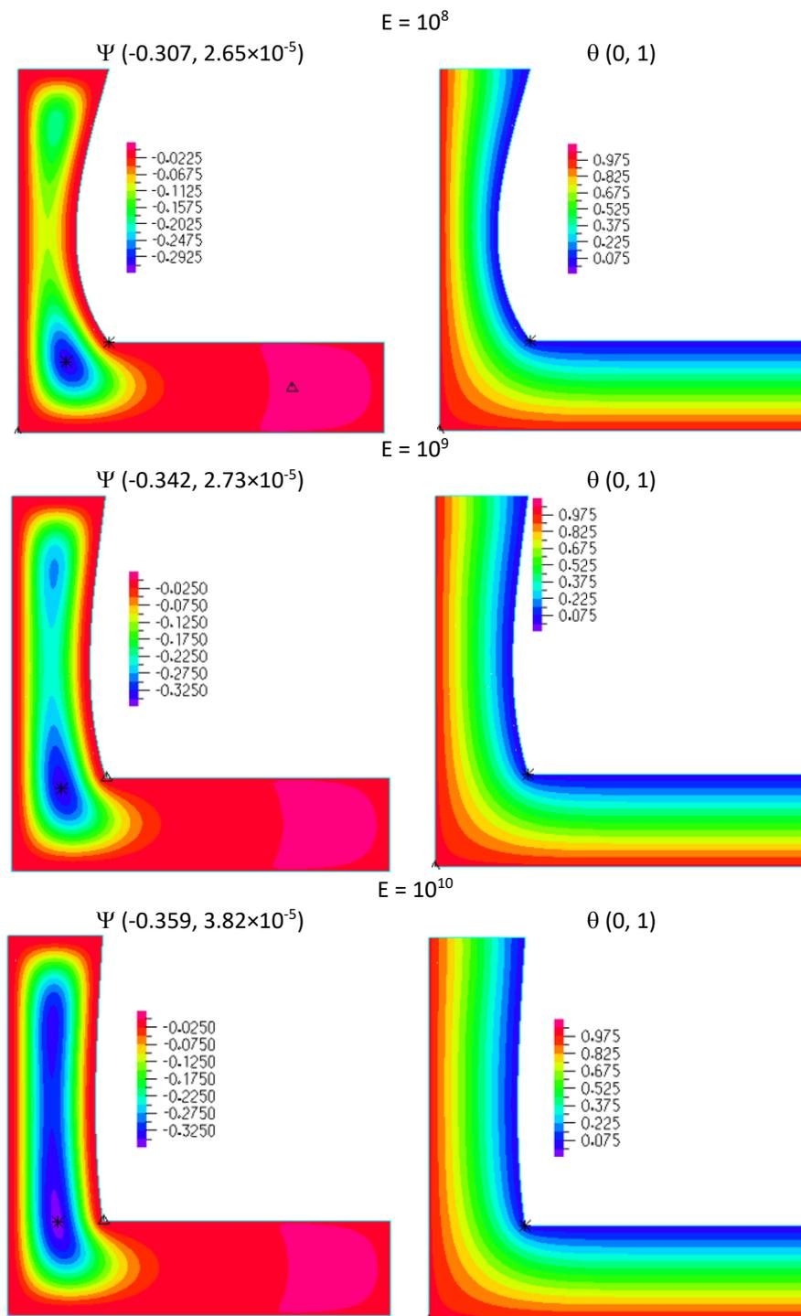
**Fig. 6.** Effect of varying the non-dimensional Young's modulus on streamlines and isotherms ( $Pr = 0.7$ ,  $Ra = 10^4$ )
