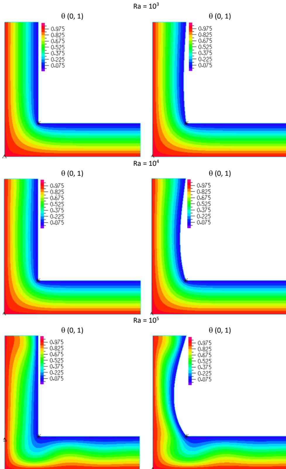
**Fig. 3.** Comparison of the isotherms between rigid and flexible wall models inside L-shaped cavity for various Rayleigh numbers ( $Pr = 0.7$ ,  $E = 10^9$ )
