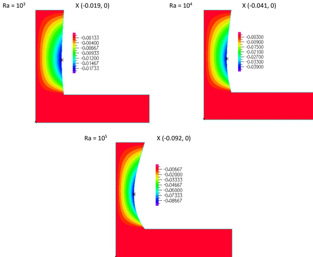
**Fig. 5.** Effect of varying Rayleigh number on X-displacement ( $Pr = 0.7, E = 10^9$ )
