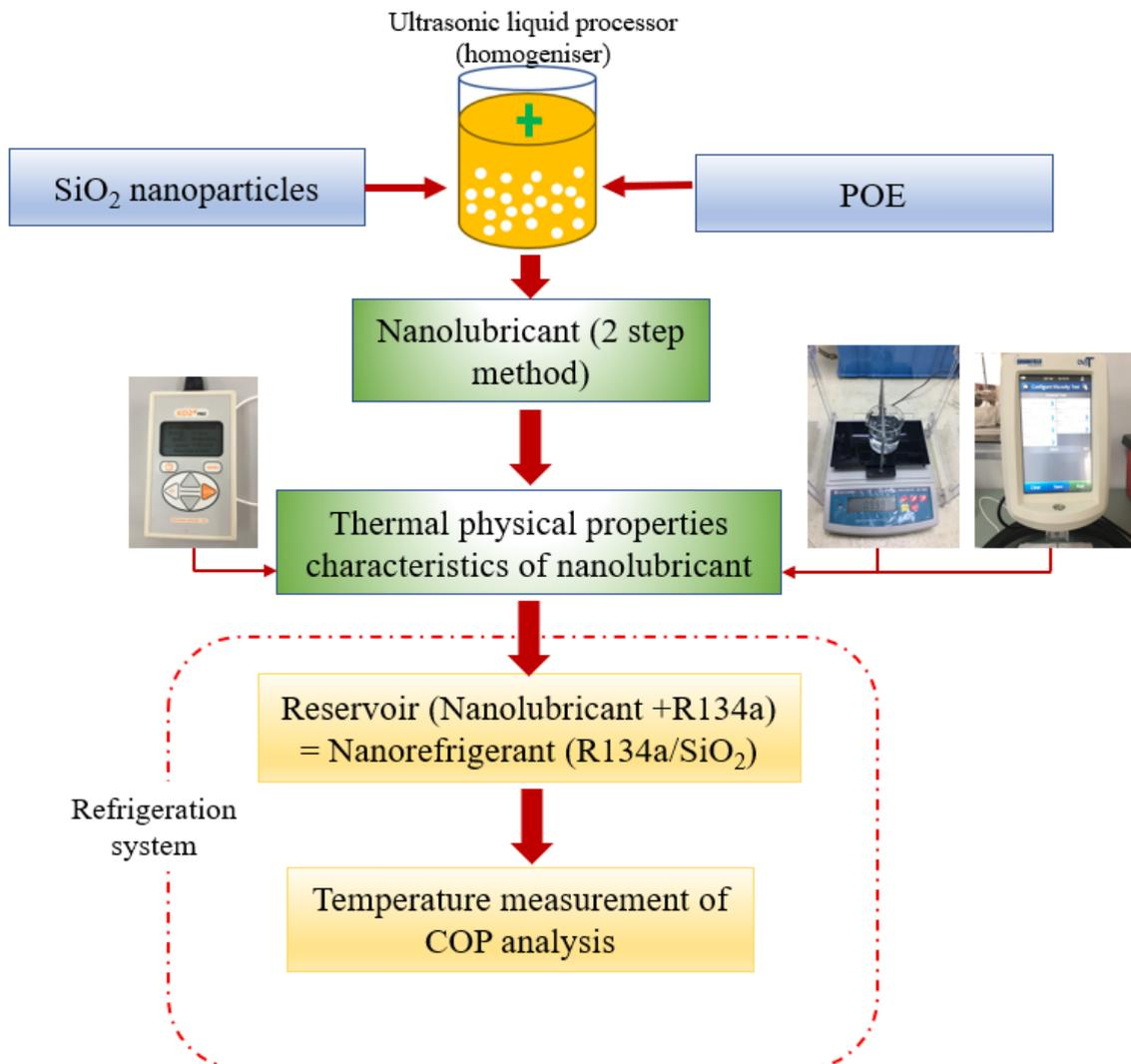
**Fig. 5.** Flow of nanolubricant and nanorefrigerant preparation and testing
