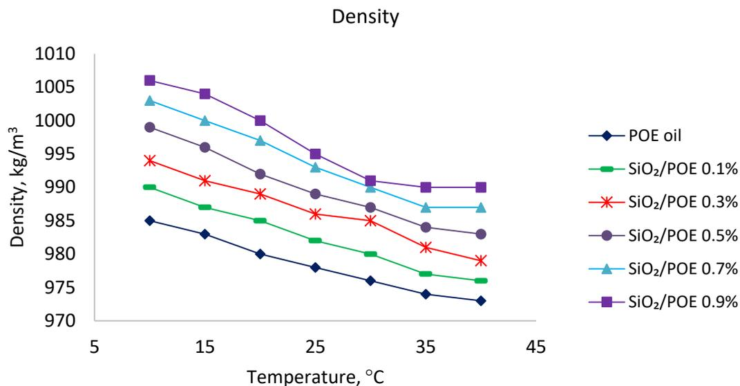
Fig. 9. Variation of density of nanolubricant with increasing temperature
