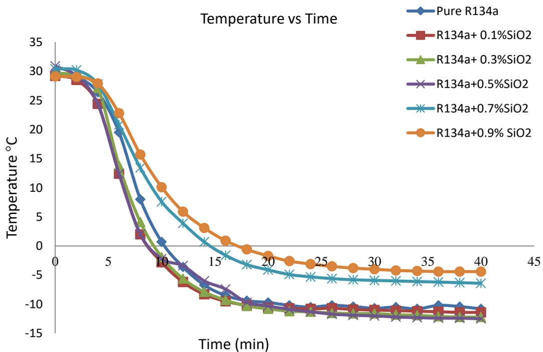
Fig. 11. Variation of temperature with time
