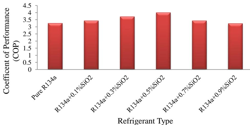
**Fig. 14.** Comparison of coefficient of performance of the six different types of refrigerants
