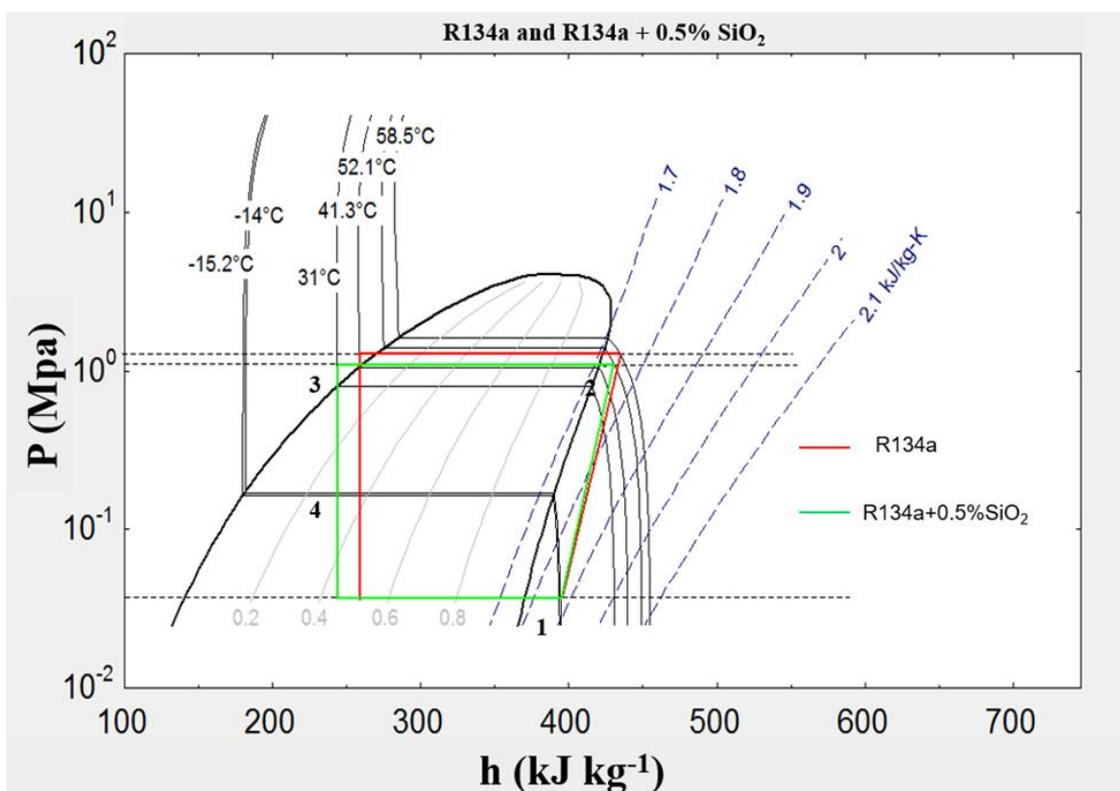
**Fig. 15.** P-h diagram of vapour compression refrigeration cycle for pure refrigerant R134a with R134a+0.5%SiO<sub>2</sub> nanorefrigerant
