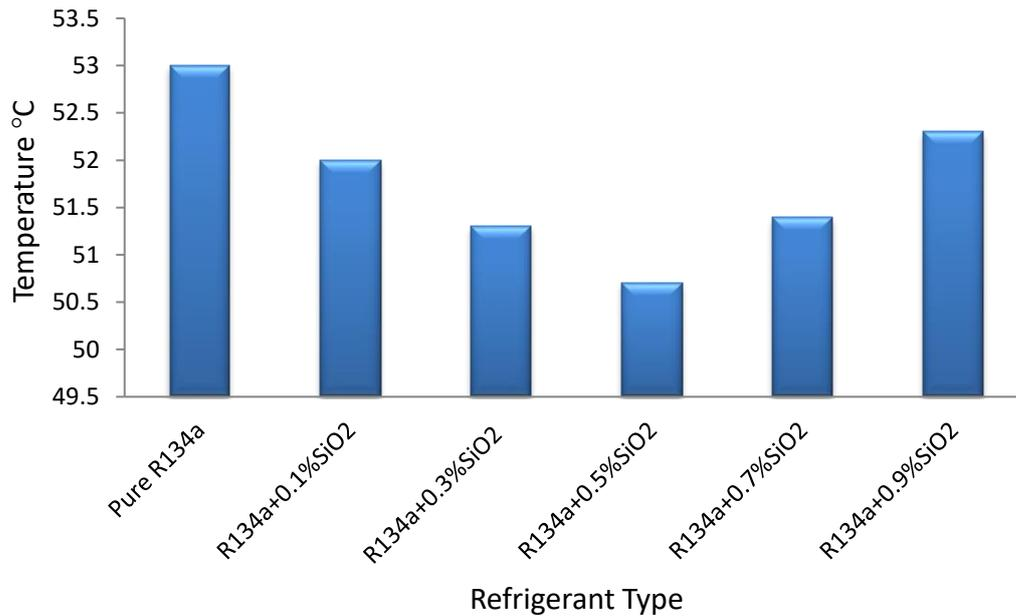
**Fig. 12.** Variations of temperature at the compressor dome
