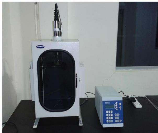
**Fig. 3.** Sonication machine for nanofluid preparation
