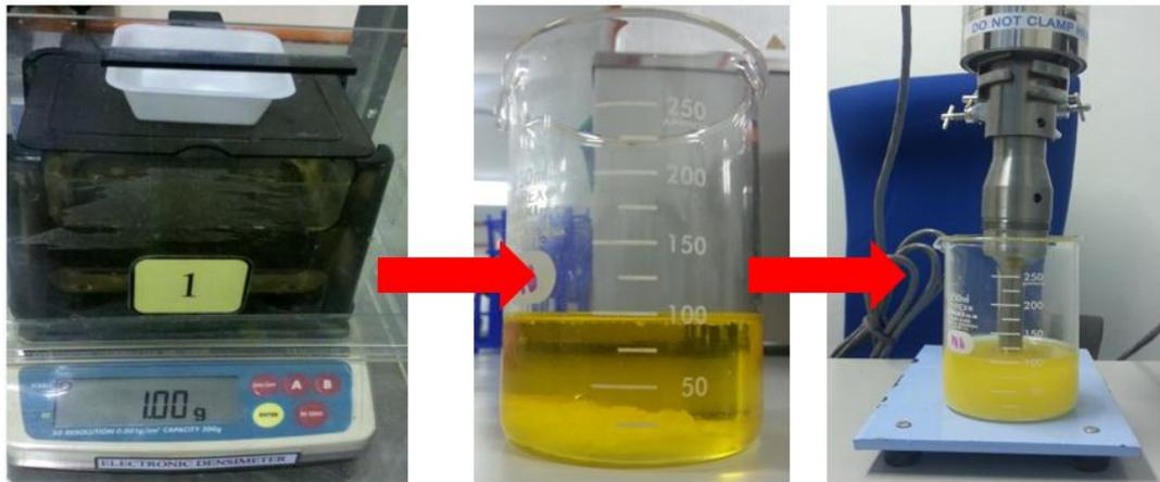
Fig. 4. Steps for nanofluid preparation
