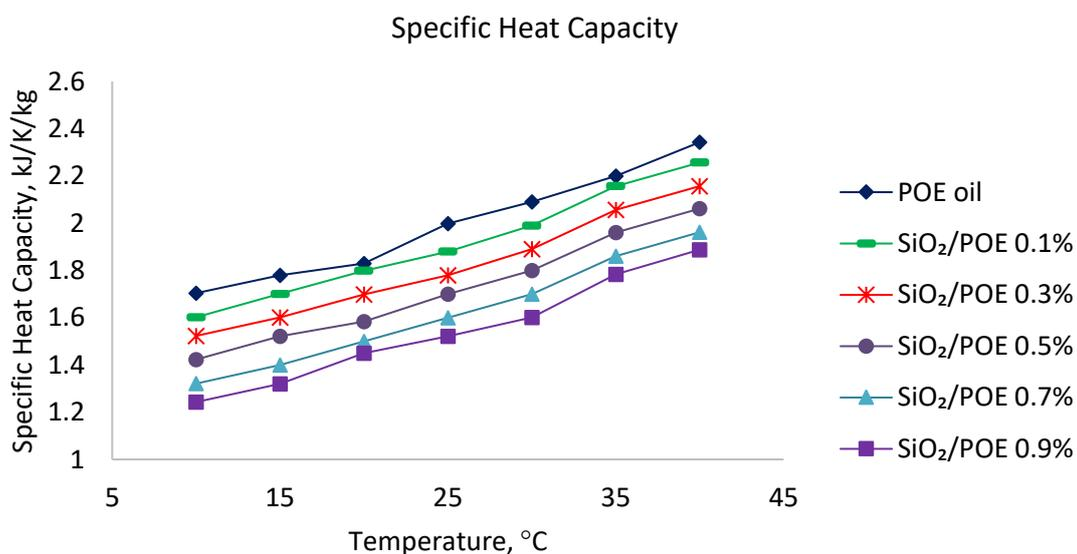
Fig. 10. Variation of specific heat capacity of nanolubricant with increasing temperature
