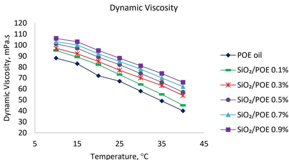
Fig. 8. Variation of dynamic viscosity of nanolubricant with increasing temperature
