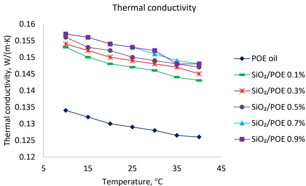
Fig. 7. Variation of thermal conductivity of nanolubricant with increasing temperature
