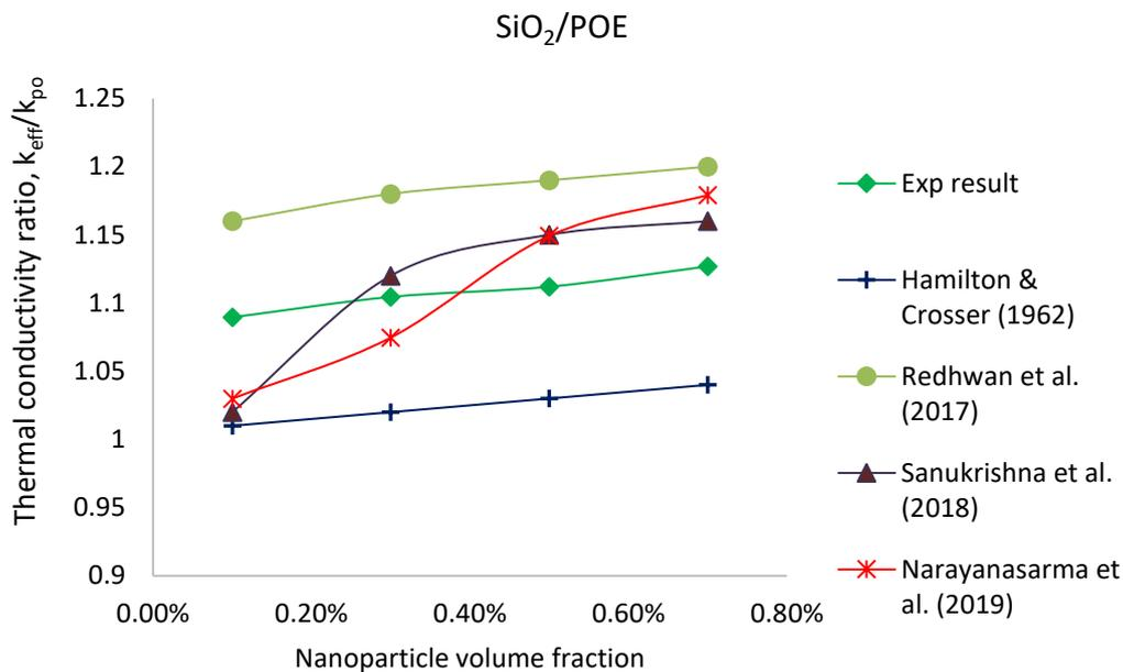
**Fig. 6.** Comparisons of thermal conductivity ratio for SiO<sub>2</sub> nanolubricant at 300 K
