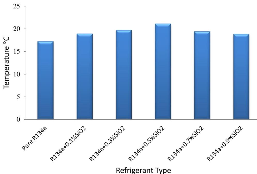
**Fig. 13.** Reduction in refrigerant temperature while passing through the condenser
