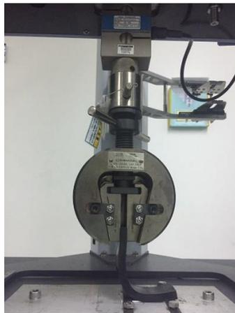
**Fig. 4.** The 90 degrees peel test performed on the rubber-metal bonding
