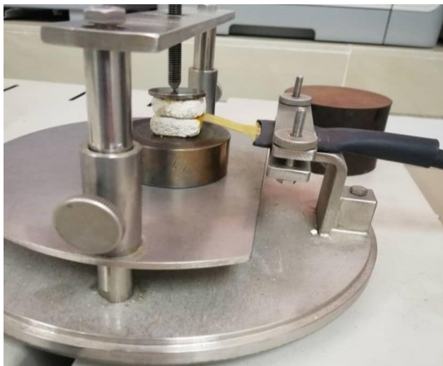
Fig. 3. Guarded hot-plate apparatus
