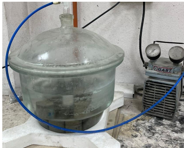
Fig. 4. Permeable porosity test
