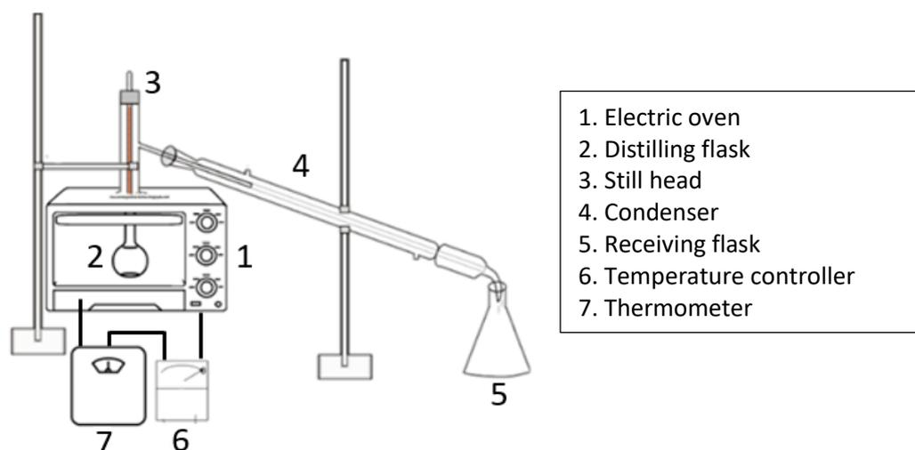
**Fig. 1.** Schematic diagram of distillation tool
