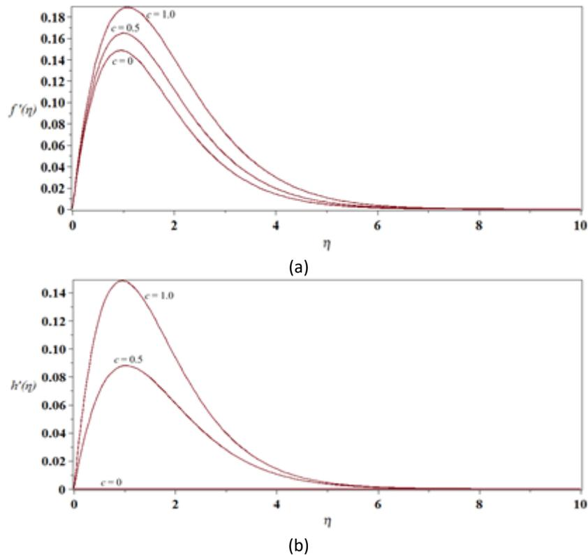
**Fig. 2.** The velocity profiles in (a)  $x$ - and (b)  $y$ -direction due to various values of the geometry ratio  $c$  at the stagnation point
