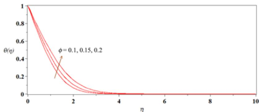
**Fig. 6.** The temperature profiles for various values of the volume fraction  $\phi$  of the hybrid nanoparticles
