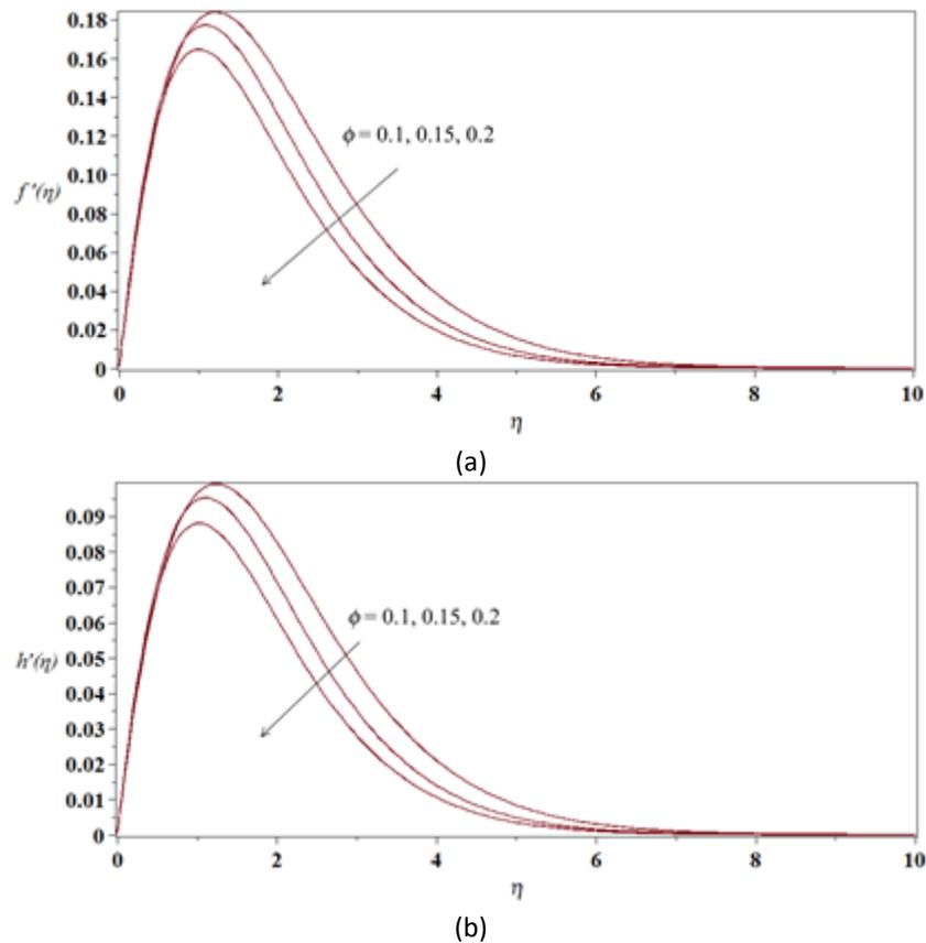
**Fig. 5.** The velocity profiles in (a)  $x$ - and (b)  $y$ -direction for various values of the volume fraction  $\phi$  of the hybrid nanoparticles
