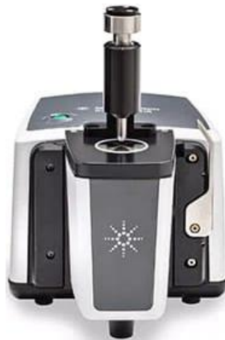
Fig. 3. Carry 630 FTIR for check sample of Zircon and Silicate nanoparticles
